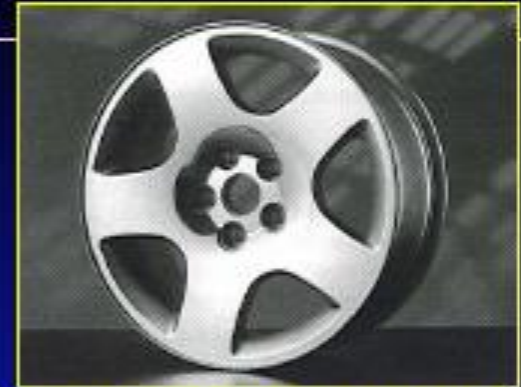
Prototype of a magnesium forged wheel(ZK30)
