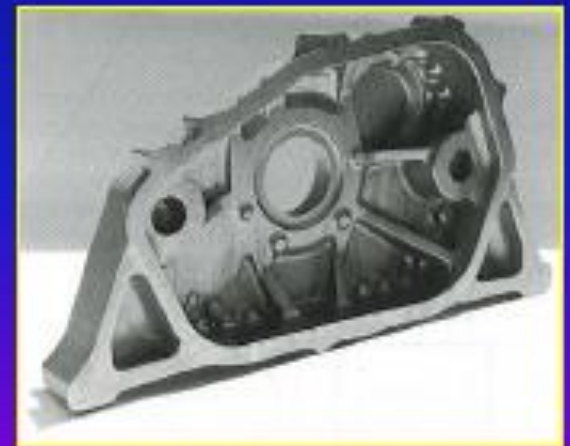
Drop-forged gearbox cover for a helicopter
