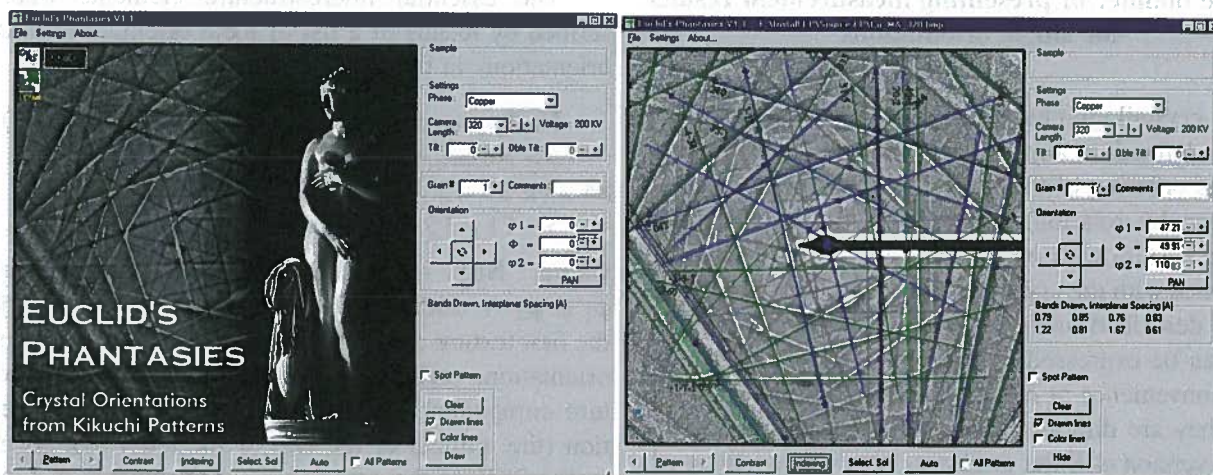
Fig. 3. The dialog box of EP software that allows one to introduce lines manually (blue lines — indicated manually, green lines — simulated image)
