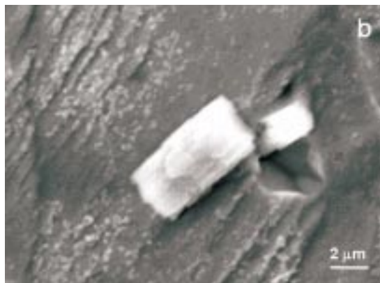
Fig. 6. Examples of a Mg-rich particle, a) TEM and b) SEM
