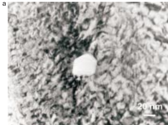
Fig. 5. TiN particles on a carbon replica
