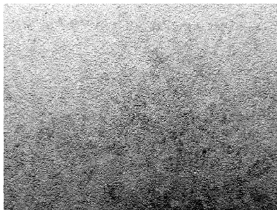
Fig. 2. Surface of Al-10wt%Si coating in initial state
