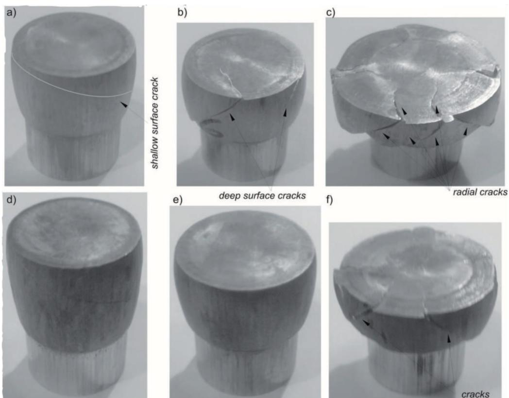
Fig. 2. Shapes of forgings made of AlCu4MgSi alloy in T42 temper (a, b, c) and in solution heat-treated state; values of mean strain  $\varepsilon$  being: -0.38 (a), -0.50 (b), -0.98 (c), -0.37 (d), -0.48 (e), -0.76 (f)
