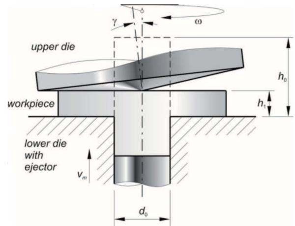
Fig. 1. Scheme of orbital forging process of forging with flange, where:  $d_0$  – original sample diameter,  $h_0$  – original height of the upset forged part of a sample,  $h_1$  – flange thickness,  $v_m$  – lower die velocity,  $\gamma$  – deflection angle,  $\omega$  – upper die orbital velocity
