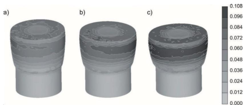
Fig. 5. Cockroft-Latham damage function distribution calculated in FEM simulation, with values of mean strain  $\varepsilon$  being: -0.36 (a), -0.43 (b) and -0.52 (c)
