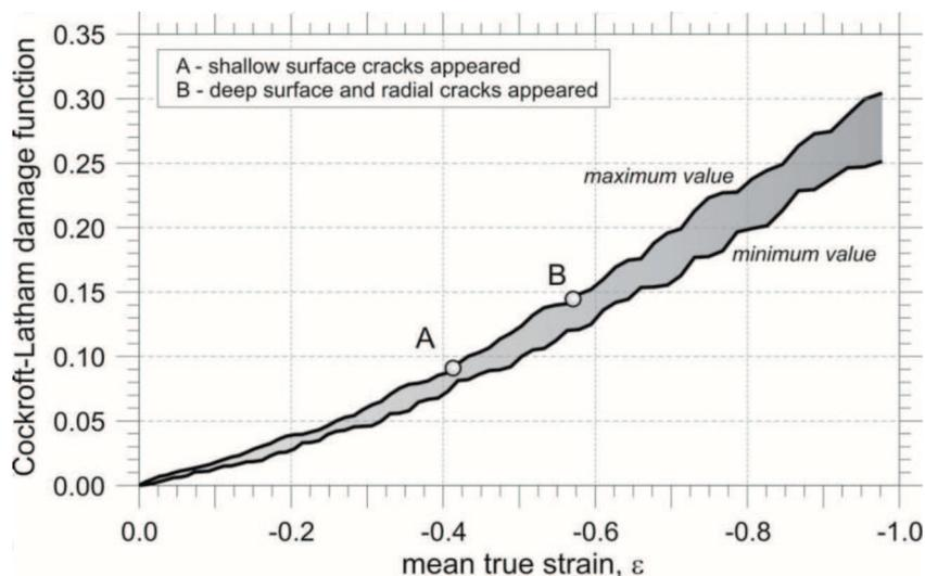
Fig. 6. Range of Cockcroft-Latham damage function values obtained in FEM simulations and calculated for flange lateral surface in the middle of thickness  $h_1$ , where: points A and B show when particular kinds of cracks appear on experimental forgings
