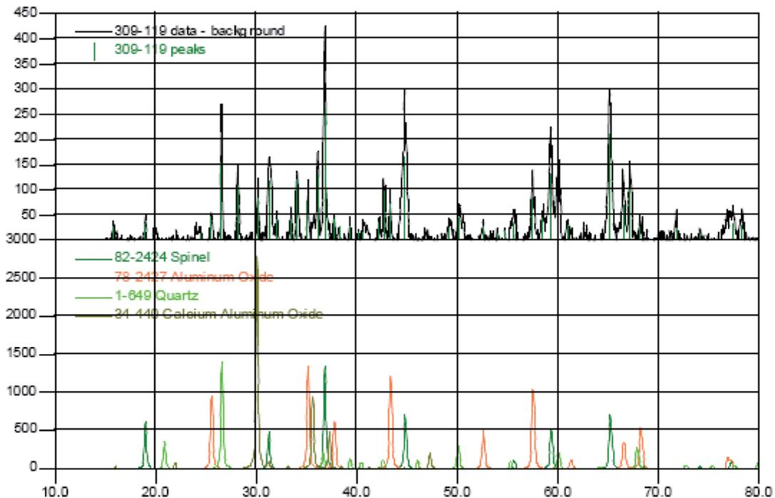
Fig. 12. The XRD diagram of the scull from the sheath tube which contains spinel,  $\text{Al}_2\text{O}_3$ ,  $\text{CaO} \cdot \text{Al}_2\text{O}_3$  and quartz
