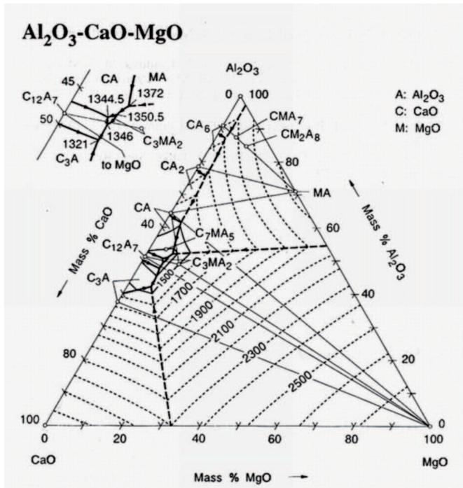
Fig. 14. The ternary system CaO- Al<sub>2</sub>O<sub>3</sub>-MgO [Slag Atlas]
