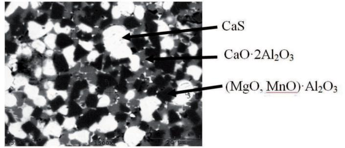
Fig. 8. The microstructure of the scull from the sheath tube with  $\text{CaS}$ ,  $\text{CaO}\cdot 2\text{Al}_2\text{O}_3$  and  $(\text{MgO, MnO})\cdot\text{Al}_2\text{O}_3$
