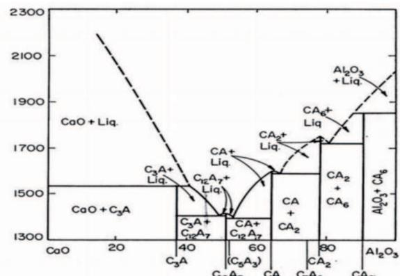
Fig. 4. Binary diagram CaO- Al<sub>2</sub>O<sub>3</sub> [6]
