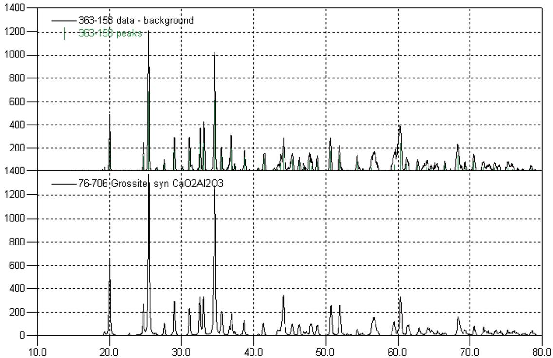
Fig. 11. The XRD diagram of the scull from the sheath tube which contains  $\text{CaO} \cdot 2\text{Al}_2\text{O}_3$
