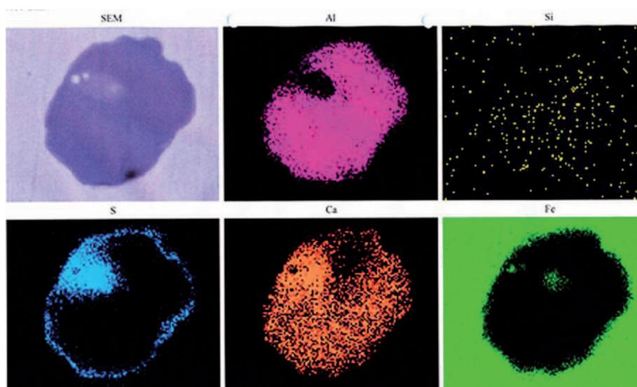
Fig. 6. Inclusions of calcium aluminate and calcium sulphide [4]
