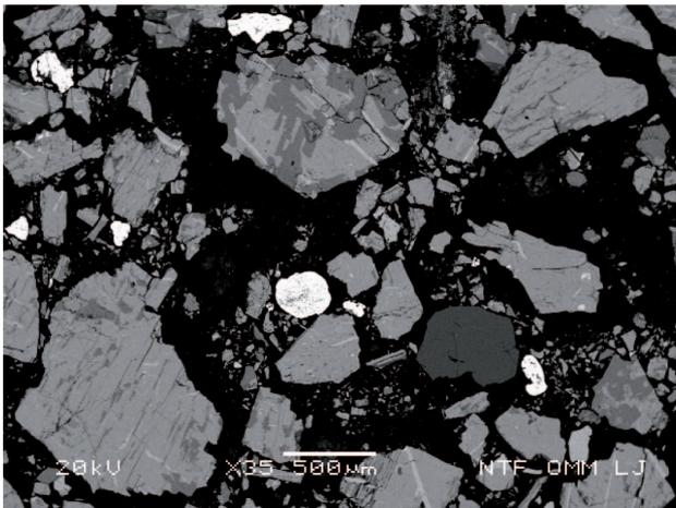
Fig. 2. Calcium silicon grain size used for injecting
