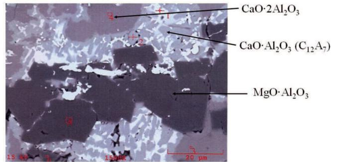
Fig. 9. The microstructure of the scull from the sheath tube
