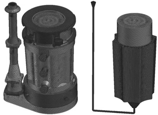
Fig. 2. View of the final computational mesh of the casting system
