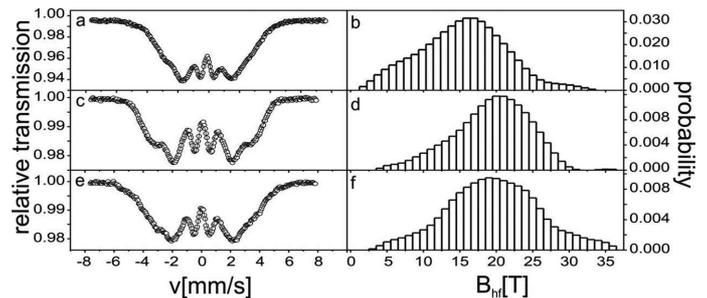
Fig. 3. Transmission Mössbauer spectra (a, b, c) and corresponding hyperfine field induction distributions (d, e, f) for amorphous powdered alloys after preparation: (a, d) – ( $\text{Fe}_{0.61}\text{Co}_{0.10}\text{Zr}_{0.025}\text{Hf}_{0.025}\text{Ti}_{0.02}\text{W}_{0.02}\text{B}_{0.20}$ )<sub>98</sub>Y<sub>2</sub>, (b, e) –  $\text{Fe}_{61}\text{Co}_{10}\text{Ti}_3\text{Y}_6\text{B}_{20}$ , (c, f) –  $\text{Fe}_{61}\text{Co}_{10}\text{Ti}_2\text{Y}_7\text{B}_{20}$
