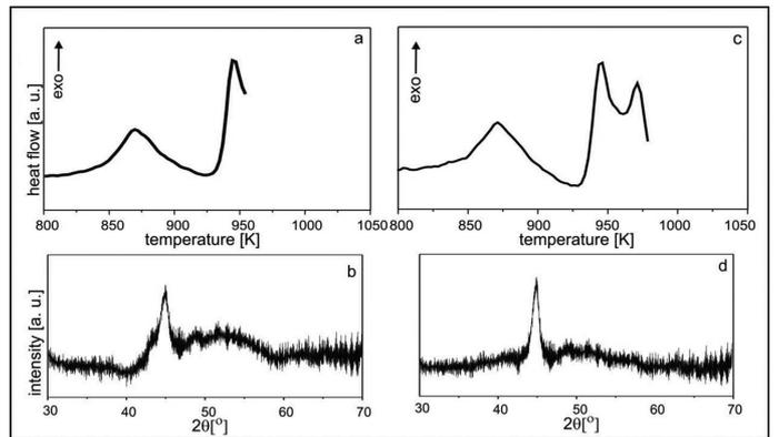
Fig. 8. DSC curves measured in the temperature range from 800 K up to 920 K (a) and from 800 K up to 1010 K (c) and X-ray diffraction patterns recorded after breaking heat treatment at 920 K (b) and 1010 K (d) for the amorphous powdered  $(\text{Fe}_{0.61}\text{Co}_{0.10}\text{Zr}_{0.025}\text{Hf}_{0.025}\text{Ti}_{0.02}\text{W}_{0.02}\text{B}_{0.20})_{98}\text{Y}_2$  alloy
