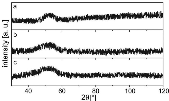
Fig. 2. XRD patterns obtained for as-received powdered samples (a) – ( $\text{Fe}_{0.61}\text{Co}_{0.10}\text{Zr}_{0.025}\text{Hf}_{0.025}\text{Ti}_{0.02}\text{W}_{0.02}\text{B}_{0.20}$ )<sub>98</sub>Y<sub>2</sub>, (b) –  $\text{Fe}_{61}\text{Co}_{10}\text{Ti}_3\text{Y}_6\text{B}_{20}$ , (c) –  $\text{Fe}_{61}\text{Co}_{10}\text{Ti}_2\text{Y}_7\text{B}_{20}$
