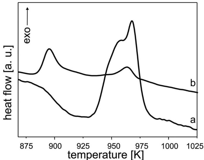
Fig. 6. Isochronal DSC curves recorded at heating rate  $10\text{ K min}^{-1}$  (a) and  $5\text{ K min}^{-1}$  (b) for the amorphous  $\text{Fe}_{61}\text{Co}_{10}\text{Ti}_3\text{Y}_6\text{B}_{20}$  alloy
