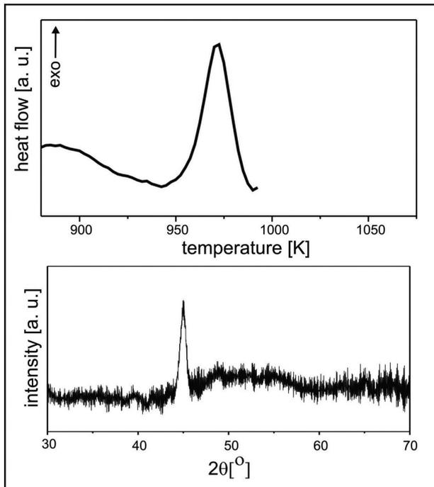
Fig. 10. DSC curve (a) measured in the temperature range from 800 K up to 990 K at the heating rate of  $10\text{ K min}^{-1}$  and X-ray diffraction pattern (b) recorded after breaking heat treatment at 990 K for the amorphous powdered  $\text{Fe}_{61}\text{Co}_{10}\text{Ti}_2\text{Y}_7\text{B}_{20}$  sample
