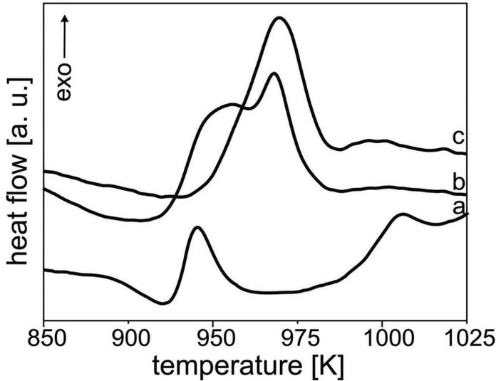
Fig. 5. DSC curves of as-received (a) –  $(\text{Fe}_{0.61}\text{Co}_{0.10}\text{Zr}_{0.25}\text{Hf}_{0.25}\text{Ti}_{0.02}\text{W}_{0.02}\text{B}_{0.20})_{98}\text{Y}_2$ , (b) –  $\text{Fe}_{61}\text{Co}_{10}\text{Ti}_3\text{Y}_6\text{B}_{20}$ , (c) –  $\text{Fe}_{61}\text{Co}_{10}\text{Ti}_2\text{Y}_7\text{B}_{20}$  alloys recorded at heating rate of  $10\text{ K min}^{-1}$
