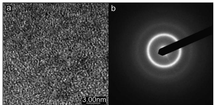
Fig. 4. Bright-field HREM-image (a) and corresponding electron diffraction pattern (b) obtained for the as-received ( $\text{Fe}_{0.61}\text{Co}_{0.10}\text{Zr}_{0.025}\text{Hf}_{0.025}\text{Ti}_{0.02}\text{W}_{0.02}\text{B}_{0.20}$ )<sub>98</sub>Y<sub>2</sub> alloy
