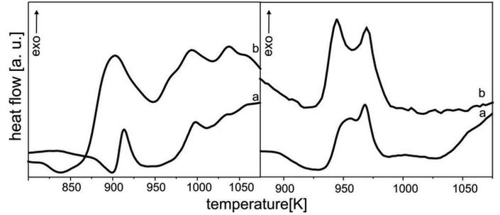
Fig. 7. DSC curves measured at the heating rate of  $10\text{ K min}^{-1}$  for the bulk amorphous (A)  $(\text{Fe}_{0.61}\text{Co}_{0.10}\text{Zr}_{0.025}\text{Hf}_{0.025}\text{Ti}_{0.02}\text{W}_{0.02}\text{B}_{0.20})_{98}\text{Y}_2$ , (B)  $\text{Fe}_{61}\text{Co}_{10}\text{Ti}_3\text{Y}_6\text{B}_{20}$ , alloys: (a) – the samples in the form of the rod; (b) – powdered rod
