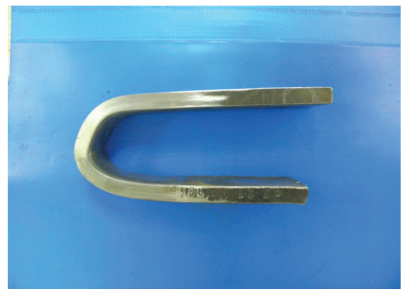
Fig. 6. A phenomena of non-axial deformation of bent samples
