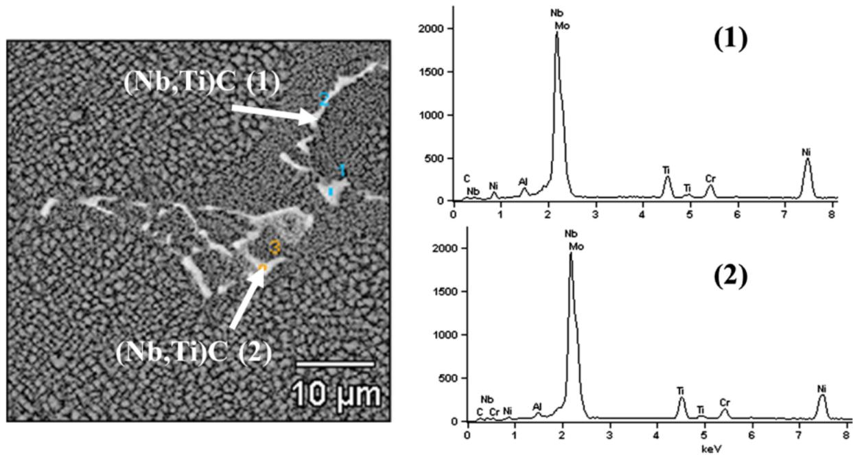
Fig. 7. The chemical and phase composition of MC carbide in IN713C superalloy HIP treatment
