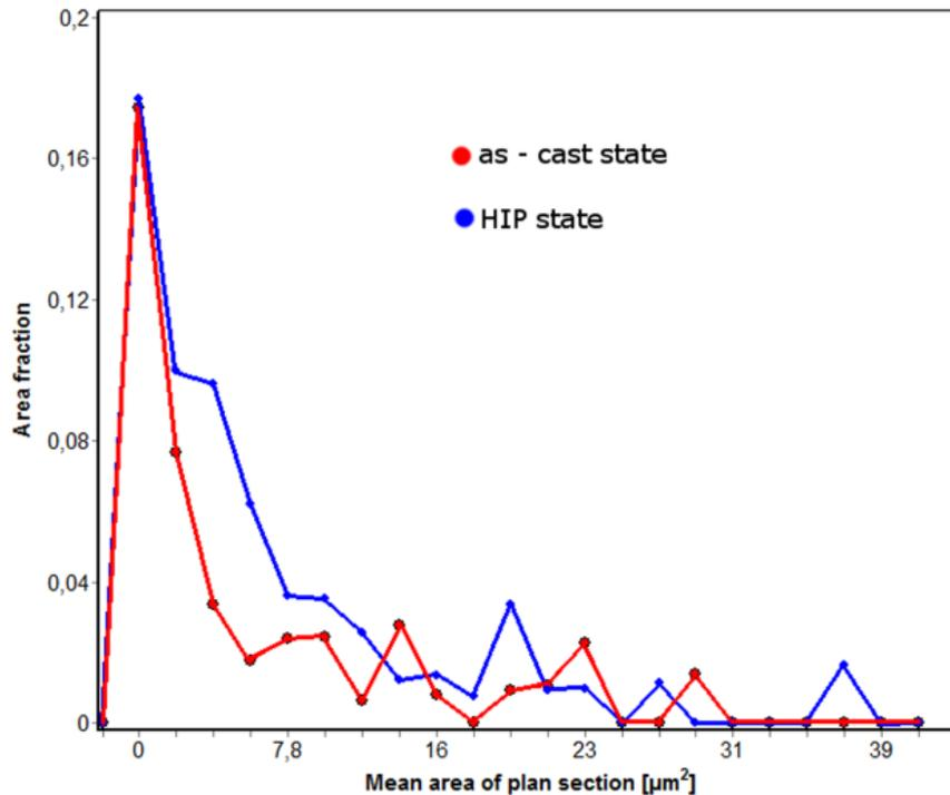
Fig. 8. Area fraction as function of plane section area of carbides in root before and after HIP
