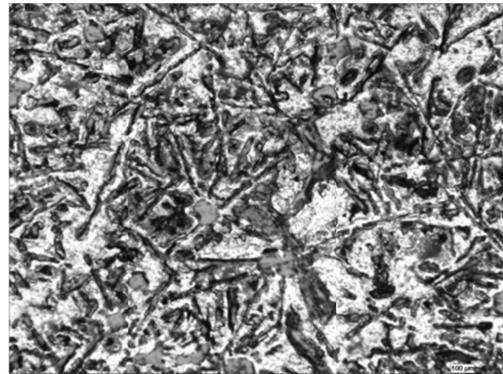
Fig. 1. Microstructure of the Base Material Al-17Si alloy
