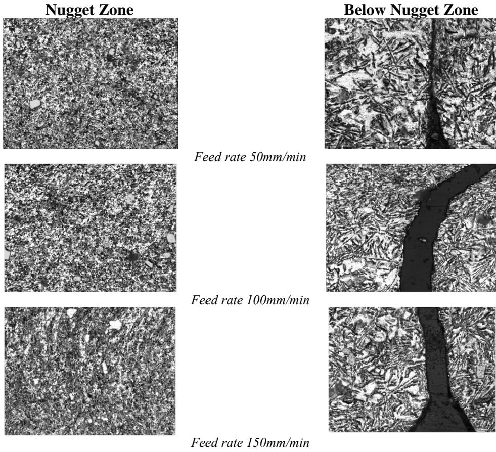
Fig. 2. Microstructure during the single pass of tool
