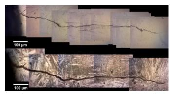
Fig. 11. Crack length developed in the specimen without charge of hydrogen (specimen type 1). a) without etching, b) with etching
