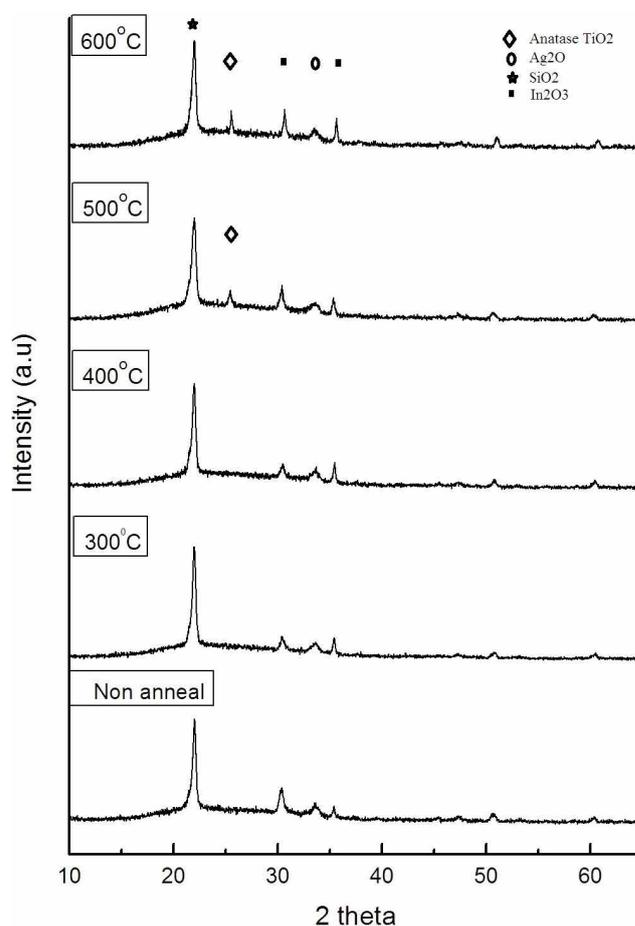
Fig. 1. XRD patterns of Ag/TiO<sub>2</sub> thin films with different annealing temperatures
