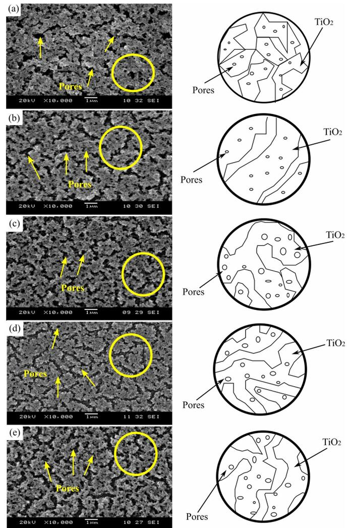
Fig. 2. SEM micrograph of Ag/TiO<sub>2</sub> thin film with different annealing temperature, (a) non-annealing, (b) 300°C, (c) 400°C, (d) 500°C and (e) 600°C
