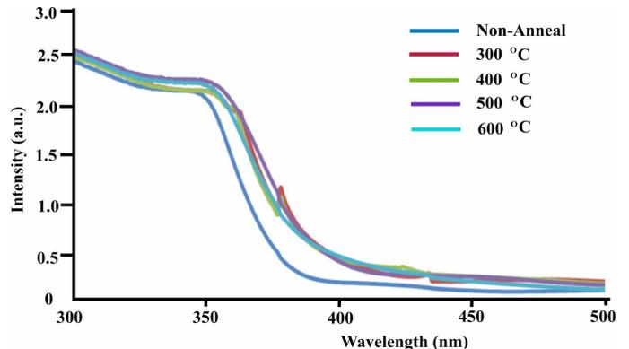
Fig. 4. Absorption curve of Ag/TiO<sub>2</sub> thin film at different annealing temperature in the spectrum range of 300 nm to 500 nm
