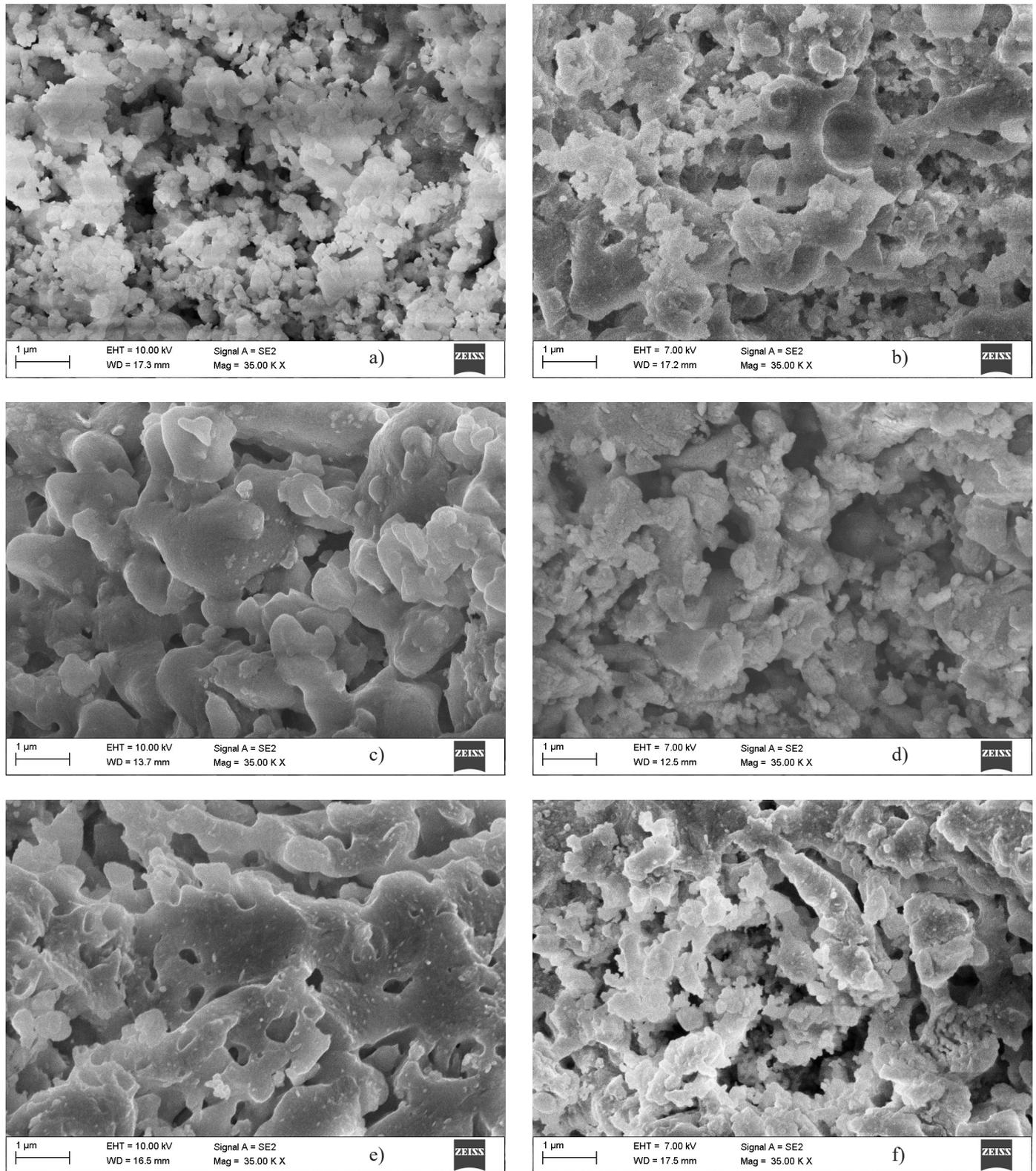
Fig. 3. Structure of fractures of porous ceramic preforms a) F40E, b) F40S, c) S40E, d) S40S, e) FS40E, f) FS40S
