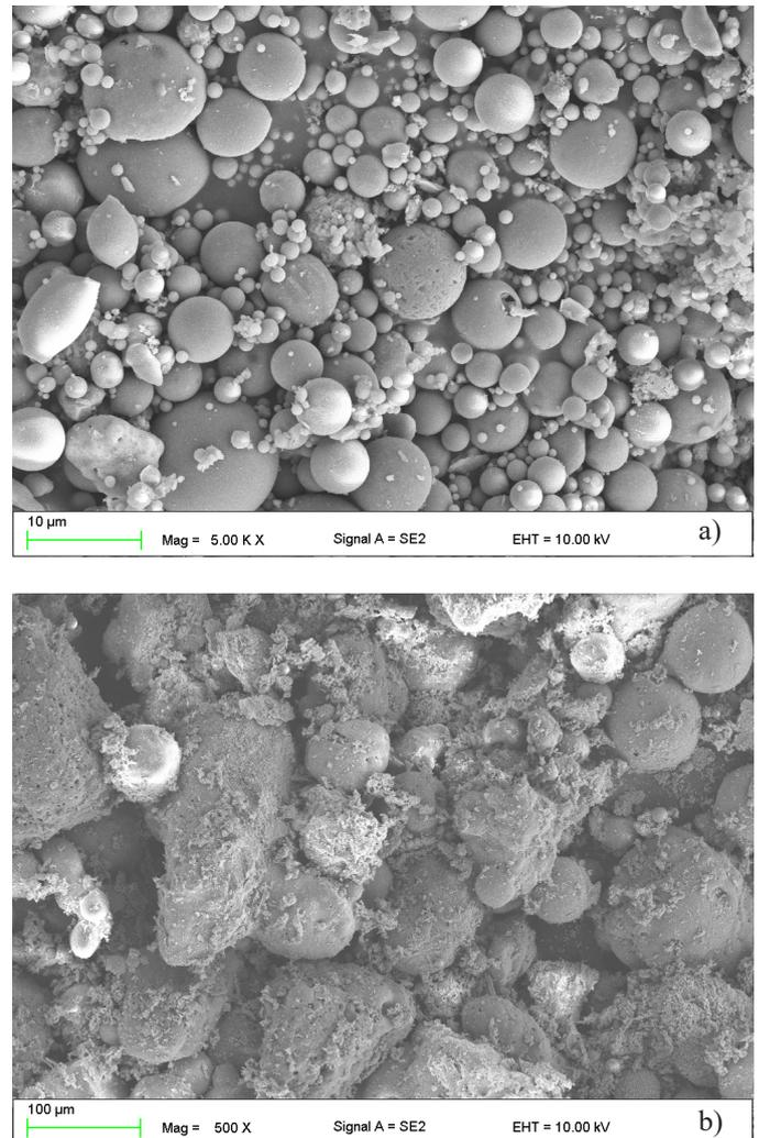
Fig. 2. Structure of coal combustion by-products: a) fly ashes, b) bottom slags
