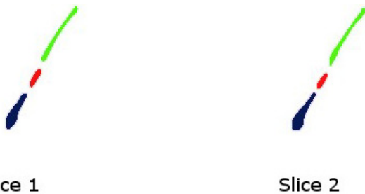
Fig. 6. Illustration of pores with the same id numbers identified on two subsequent images
