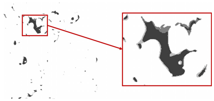
Fig. 7. Two corresponding slices (merged) with shared cells. Black cells are shared parts of each feature set, grey cells belong only to one feature
