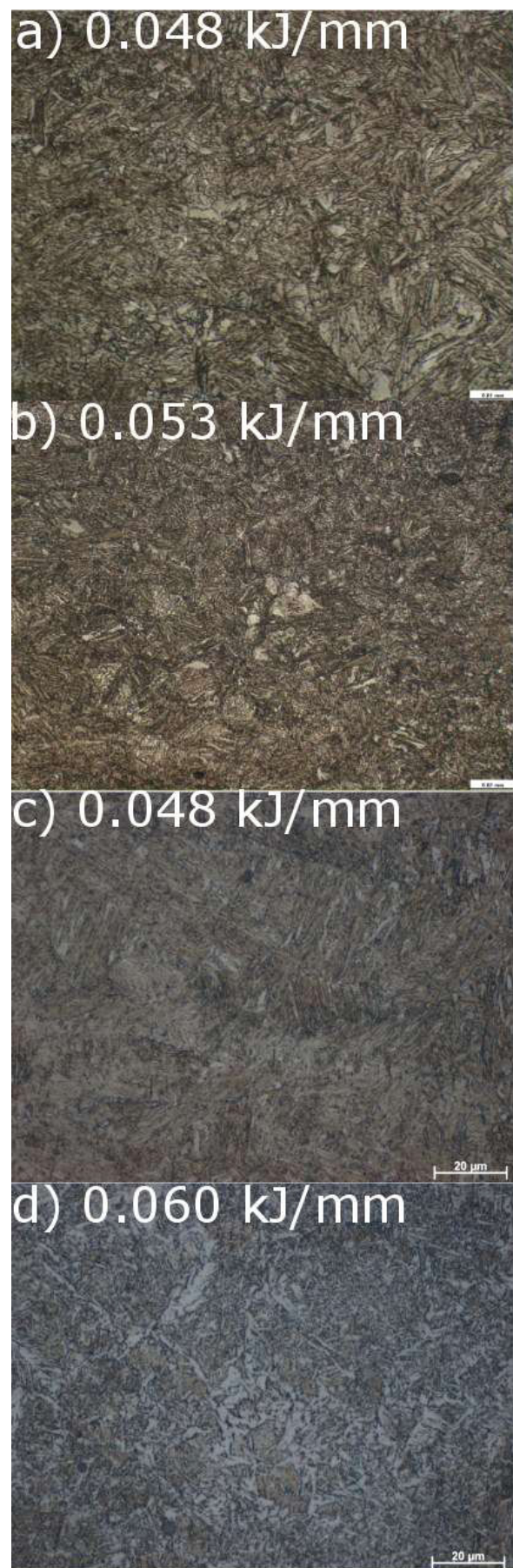
Fig. 6. Microstructure of the heat affected zone of steel TRIP subjected to: a), b) single-spot laser beam welding, c), d) twin-spot laser beam welding
