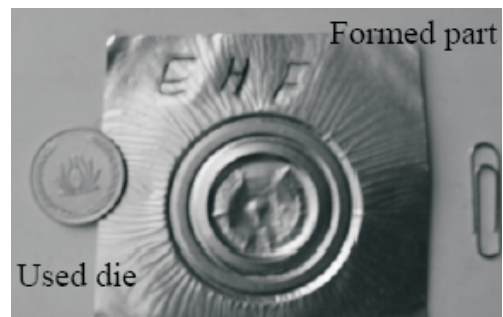
Fig. 23. Effect of entrapped air, on the product quality
