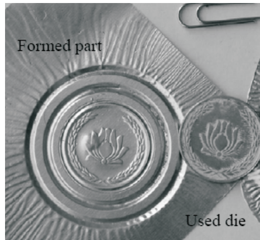
Fig. 22. Deformed precise aluminium parts made by EHF process
