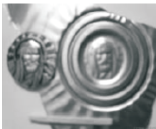
Fig. 15. Manufactured sculptural parts made by copper sheet with 0.1 thicknesses
