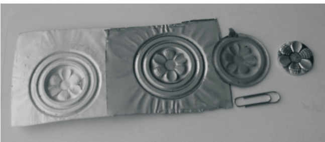
Fig. 21. Formed parts made from silver, copper and gold (left to right)
