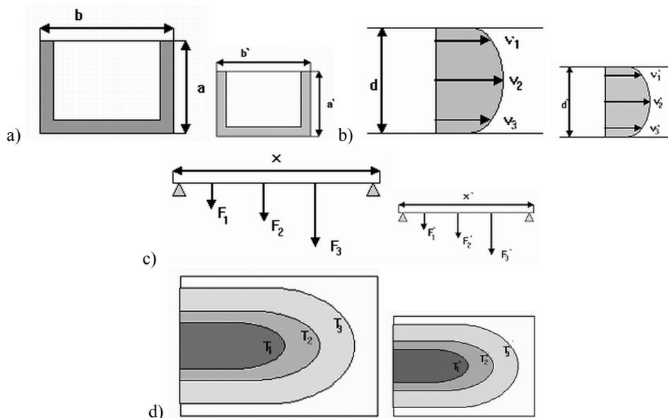
Fig. 2. The example of similarities: a) geometrical, b) kinetic, c) dynamic, d) heat one [22,23]
