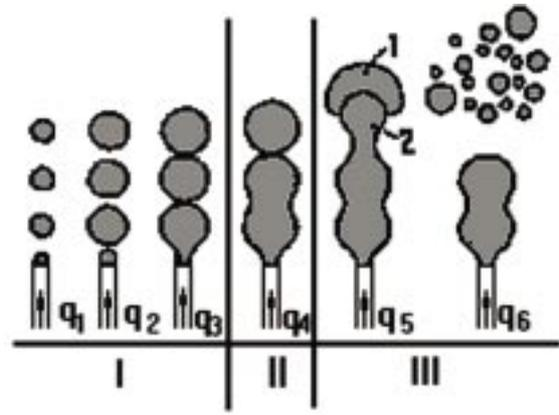
Fig. 5. The influence of the gas flow rate on the shape of gas bubbles [27]
