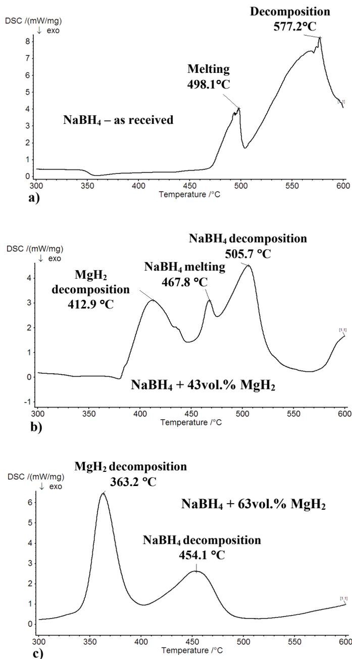
Fig. 8. DSC curves for (a)  $\text{NaBH}_4$  as-received, (b)  $\text{NaBH}_4 + 46$  vol.% $\text{MgH}_2$  and (c)  $\text{NaBH}_4 + 63$  vol.%  $\text{MgH}_2$  composites
