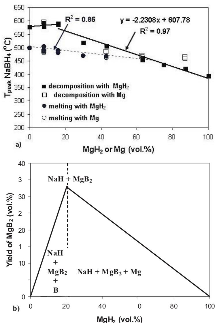
Fig. 9. The influence of  $\text{MgH}_2$  content on the destabilization of  $\text{NaBH}_4$  – (a) the  $\text{NaBH}_4$  decomposition and melting DSC peak temperatures as a function of  $\text{MgH}_2$  content; (b) The theoretical yield of  $\text{MgB}_2$  formation for  $\text{NaBH}_4 + \text{MgH}_2$  reaction as a function of  $\text{MgH}_2$  content. Adopted from [5]
