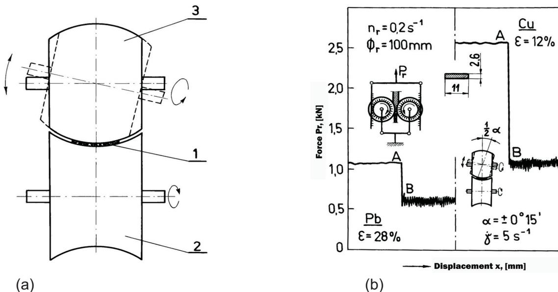
Fig. 4. Scheme of rolling with upgraded KoBo method: 1) rolled material, 2) “reel” roll, 3) swinging spherical roll (a) and the comparison of deformation force  $P_r$  in a model of rolling of lead and copper strips using conventional method “A” and KoBo one “B” (b)
