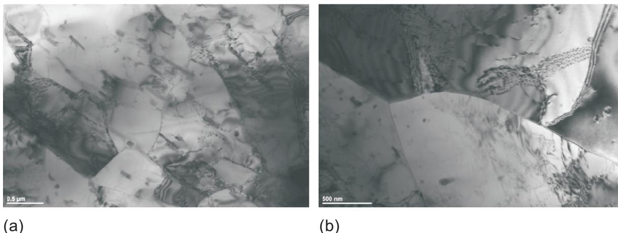
Fig. 14. Microstructures (TEM) of 7075 aluminum alloy strips supersaturated from the temperature 475° after 1h of annealing, rolled with 20% strain and naturally aged: a) rolling with KoBo method (variant marked II/A/0.5/N), b) conventional rolling (II/B/0.5/N)
