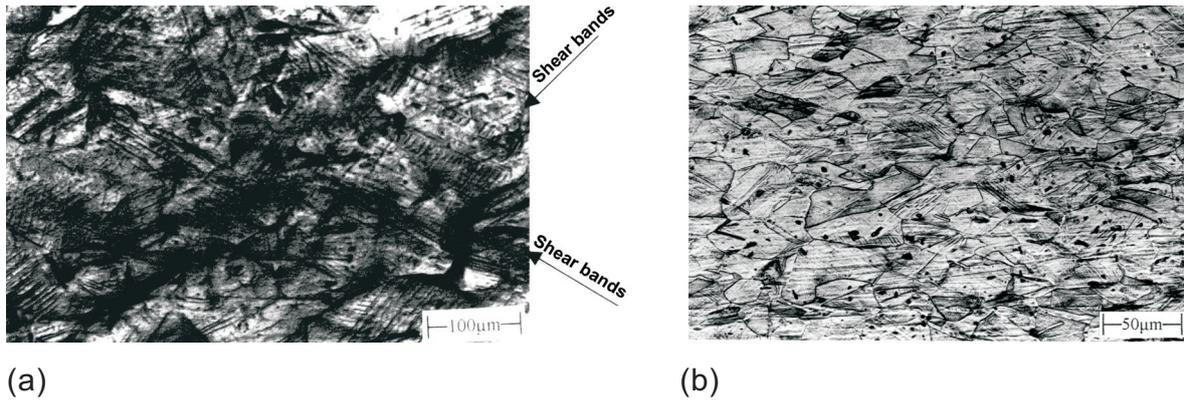
Fig. 7. Side surface topography with traces of shear bands in copper sample rolled with Cyclicform method with 6% strain (a) and the results of identical observation of copper sample rolled conventionally with 10% strain (b)
