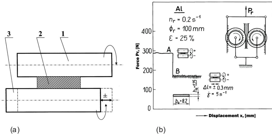
Fig. 3. Scheme of rolling with the KoBo method: 1) upper working roll, 2) rolled material (strip), 3) lower working roll cyclically-moving along its axis (a) and comparison of deformation force  $P_r$  in a model of aluminum rolling using conventional “A” and KoBo “B” method (b)
