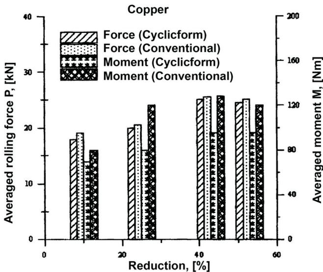
Fig. 6. Comparison of the average values of rolling force P and
