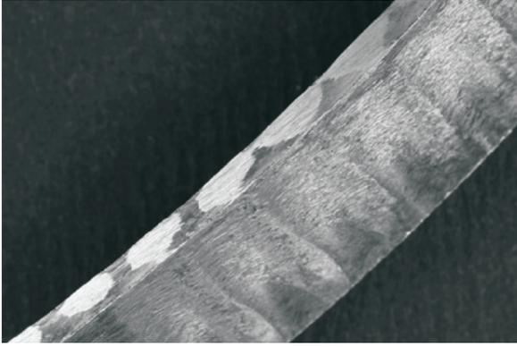
Fig. 11. View of 7075 aluminum alloy strip after rolling in accordance with variant A, using the research stand presented in Fig. 9b
