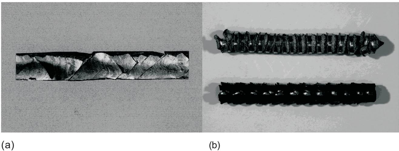
Fig. 2. Results of intense localization of deformation visible in the defective products received in the plastic deformation processes: a) side surface of the rolled CuZn37 brass tape, b) a view of conventionally extruded 7075 aluminium alloy (upper sample) and a mixture of Cu+5%  $\text{Al}_2\text{O}_3$  powders.
