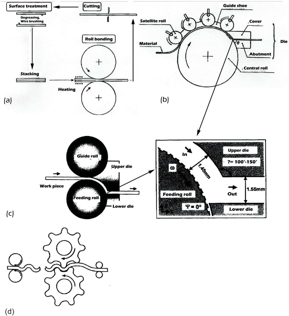
Fig. 1. Methods of continuous rolling: a) ARB [20], b) and c) C2S2 [22,23], d) cRCS [24]
