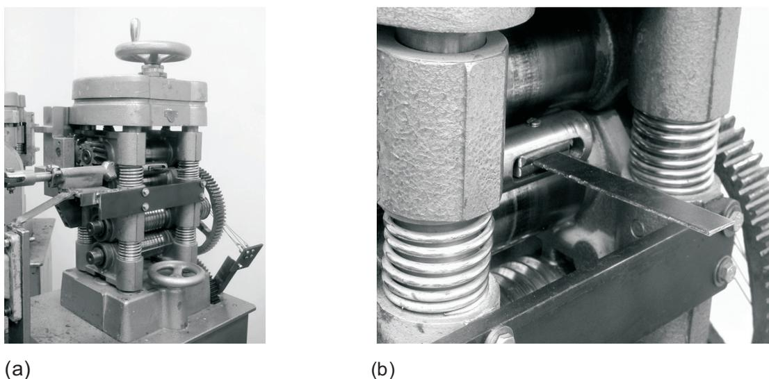
Fig. 10. Research stand designed for rolling of materials (strips) with cyclic change of inserting angle of the material between the rolls (as in Fig. 9b): a) general view, b) view of the rolling adapter (cyclic shifted frame with swinging element)
