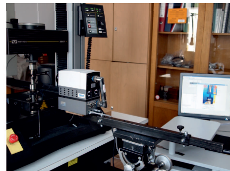
Fig. 1. Diagram and photograph of the experimental set up applied for investigation of mechanical and temperature characteristics of the FSMA loaded in compression test
