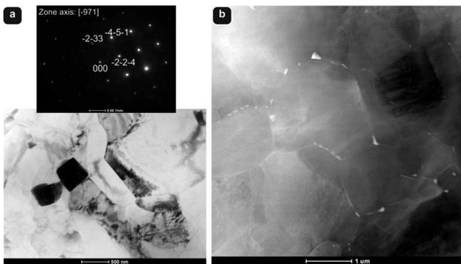
Fig. 7. The microstructure of the Mg-2.5%Tb-0.78%Sm alloy after 4 passes of ECAP at 350°C (with according to "I" procedure): (a) the TEM bright-field image of grain structure and SADP of the  $Mg_{24}(Tb,Sm)_5$  particle, (b) STEM HAADF image
