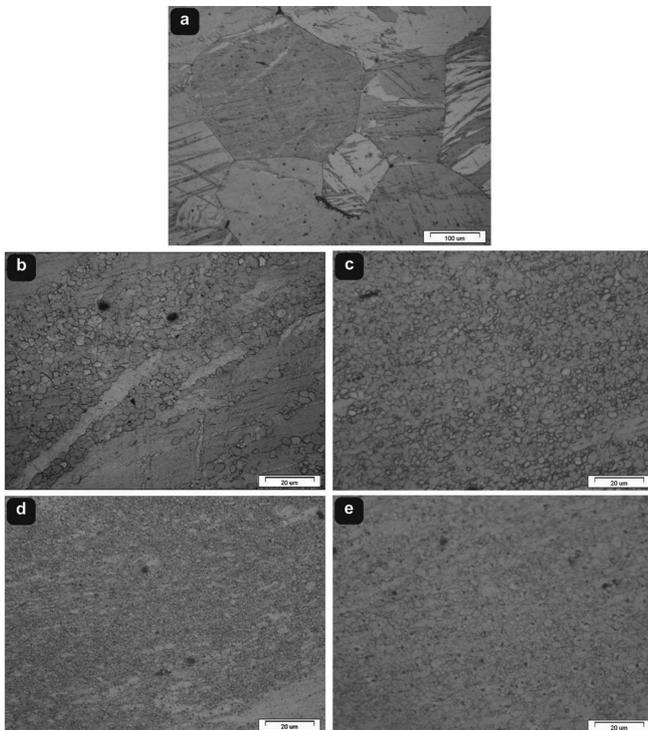
Fig. 3. The grain structure development of the Mg-2.5%Tb-0.78%Sm alloy during ECAP: (a) as rolled at 450°C – the initial structural state of the billets before ECAP, (b) after single pass at 350°C, (c) after one pass at 370°C and second at 340°C, (d) after one pass at 370°C, second at 340°C and third at 370°C – "II" procedure, (e) after four passes at 350°C – "I" procedure
