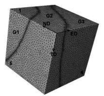
Fig. 3. The FE mesh reflecting morphology of grains of the real specimen. The mesh is finer on grain boundaries and coarser in bulk material
