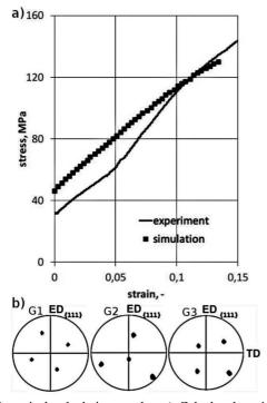
Fig. 4. Numerical calculation results: a) Calculated strain – stress curve reffered to experimental data; b) Calculated pole figures for grains G1, G2 and G3
