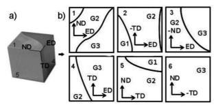
Fig. 1. a) The specimen composed of three grains prepared for compression test, b) grain boundaries schematically depicted for each side of the specimen
