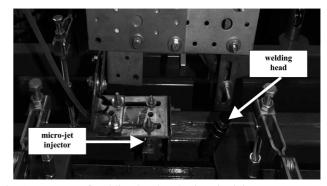
Fig. 1. Montage of welding head and micro-jet injector
