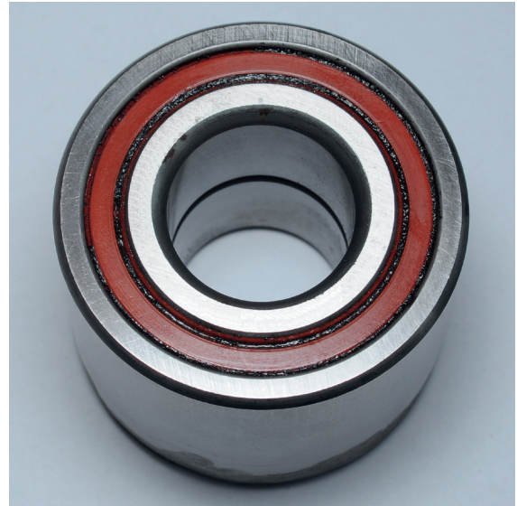
Fig. 3. Bearing VKBA 3692 from wheel of Renault Kangoo
