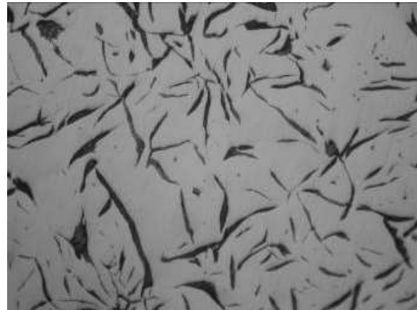
Fig. 15. Microstructure of cast iron carburized with synthetic graphite mag. 200x
