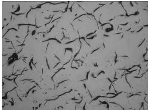
Fig. 13. Microstructure of cast iron carburized with natural graphite mag. 200x
