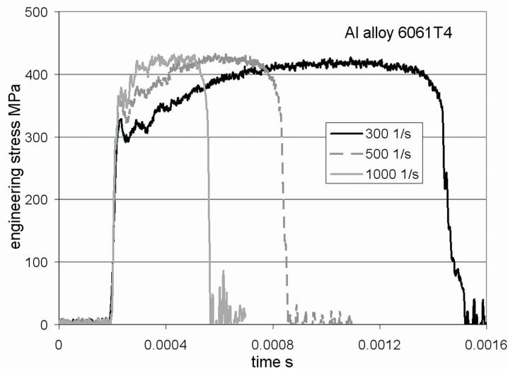
Fig. 7. Tensile curves of aluminum alloy 6061T4 for testing strain rates
