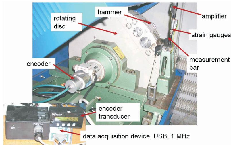
Fig. 2. Rotating hammer with a measurement system
