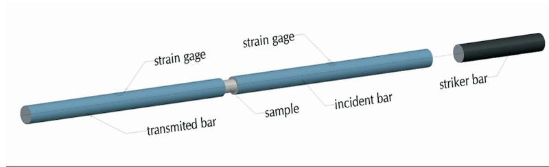
Fig. 1. General idea of splitting Hopkinson bar measurement system (SHPB) for compression tests
