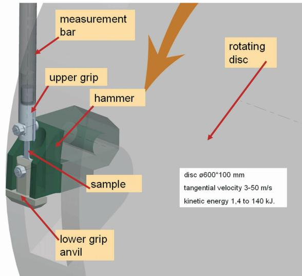
Fig. 3. Rotating disc as a hammer
