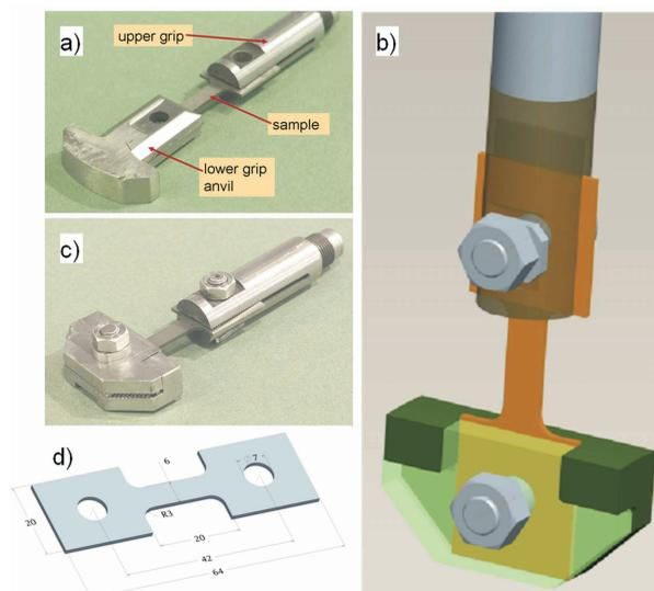
Fig. 4. Grips and a sample used during testing: a – upper grip and long lower grip, b and c – short, universal grip, d – sample
