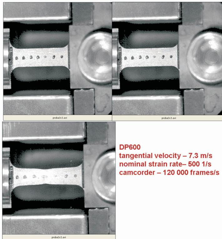
Fig. 13. Example of frames recorded by the fast camcorder
