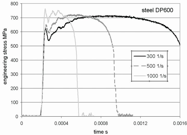
Fig. 6. Tensile curves of steel DP600 for testing strain rates
