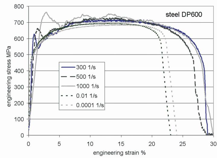
Fig. 9. Stress strain curves of steel DP600 for quasi-static and dynamic strain rates
