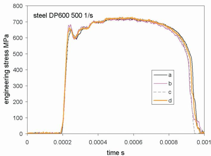
Fig. 5. Tensile curves of steel DP600, strain rate – 500 1/s
