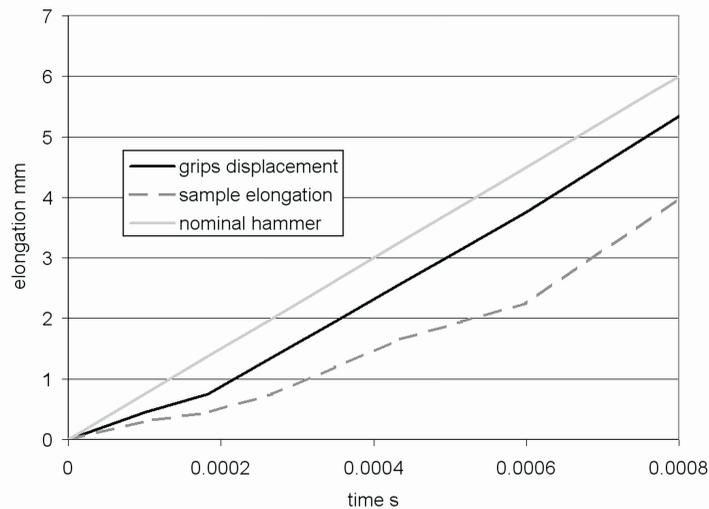
Fig. 14. The nominal hammer displacement, relative grips displacement and elongation of the sample gage length
