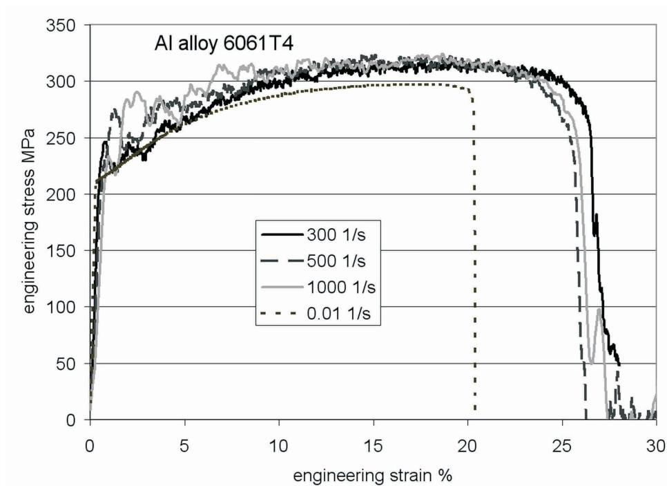
Fig. 11. Stress strain curves of aluminum alloy 6061T4 for quasi-static and dynamic strain rates
