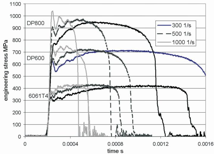
Fig. 8. Tensile curves of tested materials for testing strain rates
