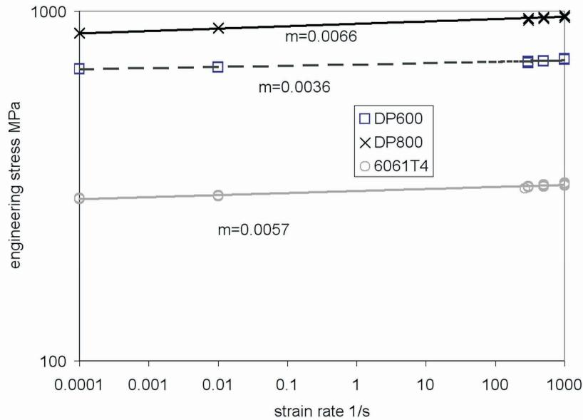
Fig. 12. The effect of strain rate on the engineering stress
