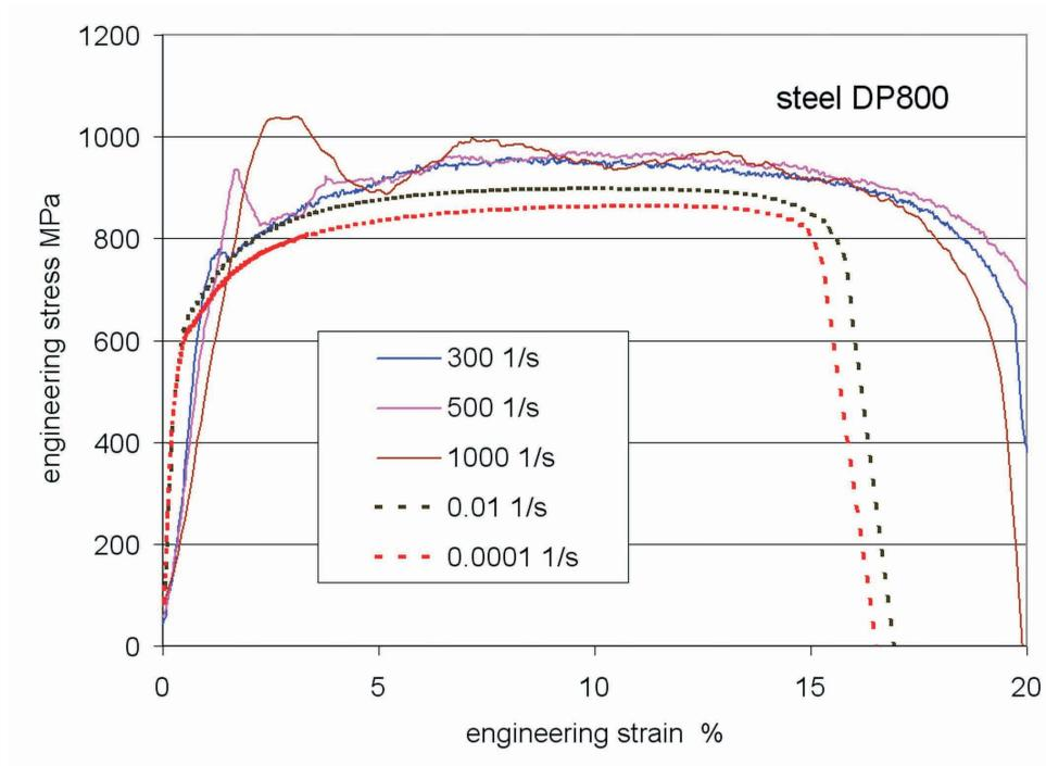
Fig. 10. Stress strain curves of steel DP800 for quasi-static and dynamic strain rates
