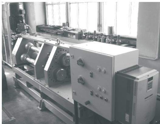
Fig. 4. The formed part in the workspace of prototype machine for rolling – extrusion process
