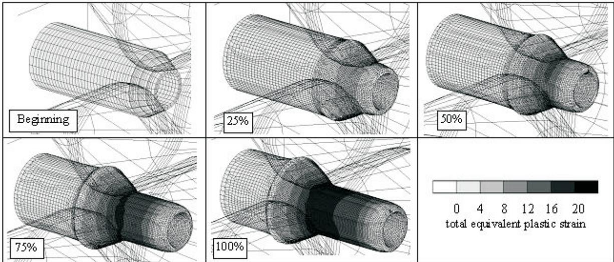
Fig. 2. Distribution of strains and progression of shape of hollowed part during rolling -extrusion process at:  $\alpha=35^{\circ}$ ,  $L=12\text{ mm}$  and  $p=5\text{ mm/rot.}$
