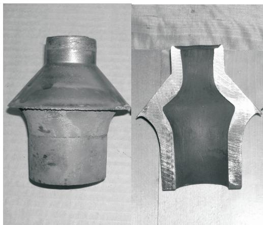
Fig. 5. An example of hollowed part obtained in rolling – extrusion
