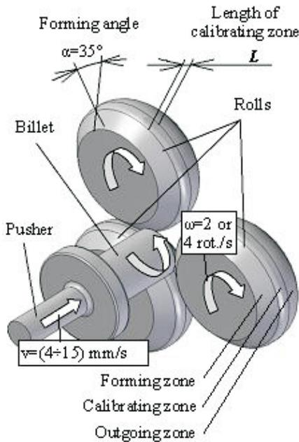
Fig. 1. Schema of rolling – extrusion process with description of tools/billet movements and basic process parameters
