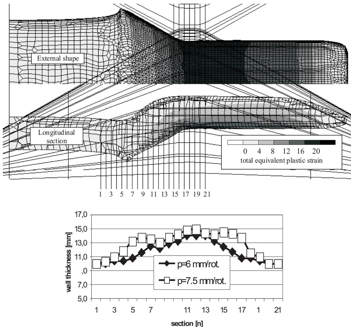
Fig. 3. The external shape and longitudinal section of hollowed parts with distribution of wall thickness at different feed rates
