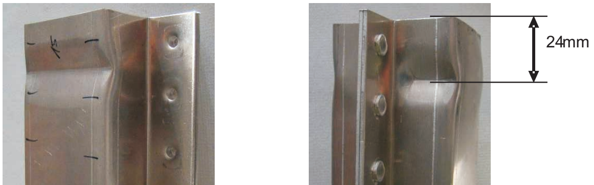
Fig. 11. Prestamping of thin-walled section on ram side (introduction of imperfections)
