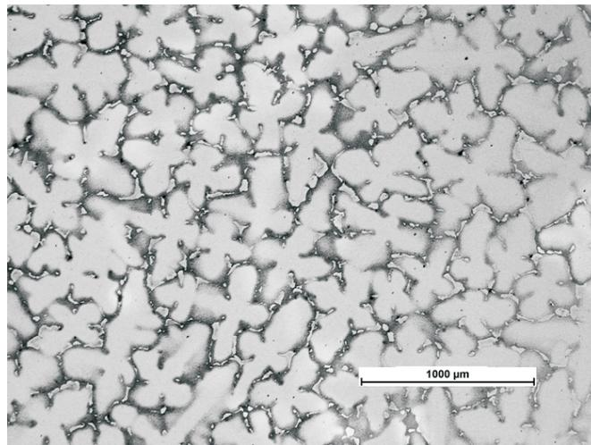
Fig. 9. The microstructure of CMSX-6 single crystal turbine blade (area before grain selector of the turbine blade)
