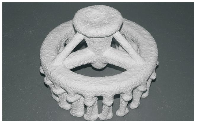
Fig. 2. Ceramic modul for production the single crystal turbine blades
