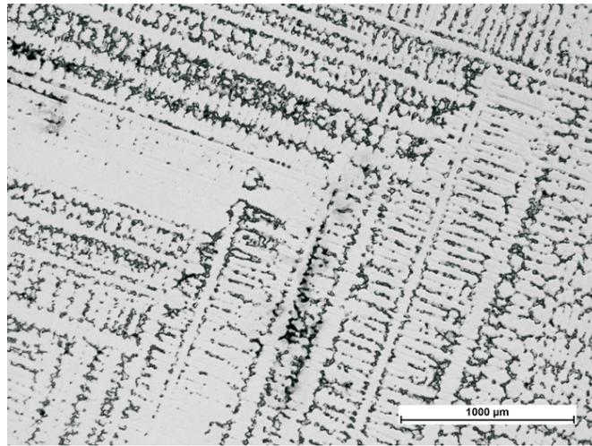
Fig. 8. The microstructure of CMSX-6 single crystal turbine blade (last area of the turbine blade)
