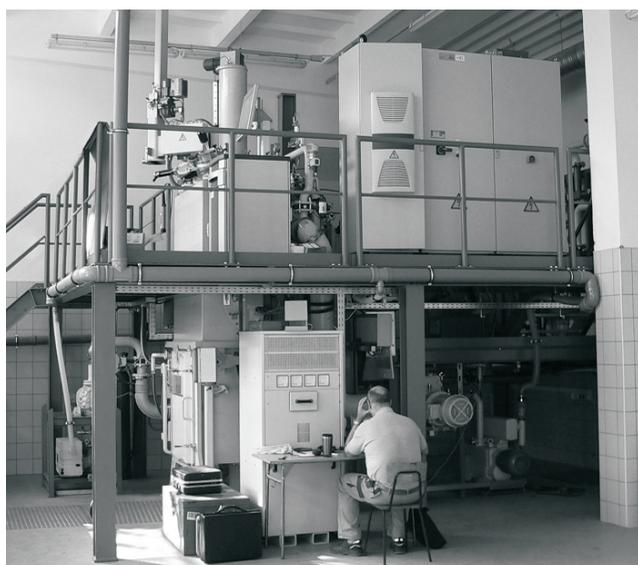
Fig. 3. Vacuum Induction Melting furnace ALD for investment casting of single crystal materials
