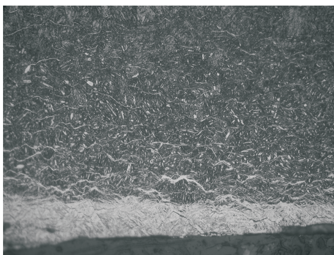
Fig. 3. Microstructure of nitrided layer – sample N° 1A etched with \text{MnFe} , mag. x500
