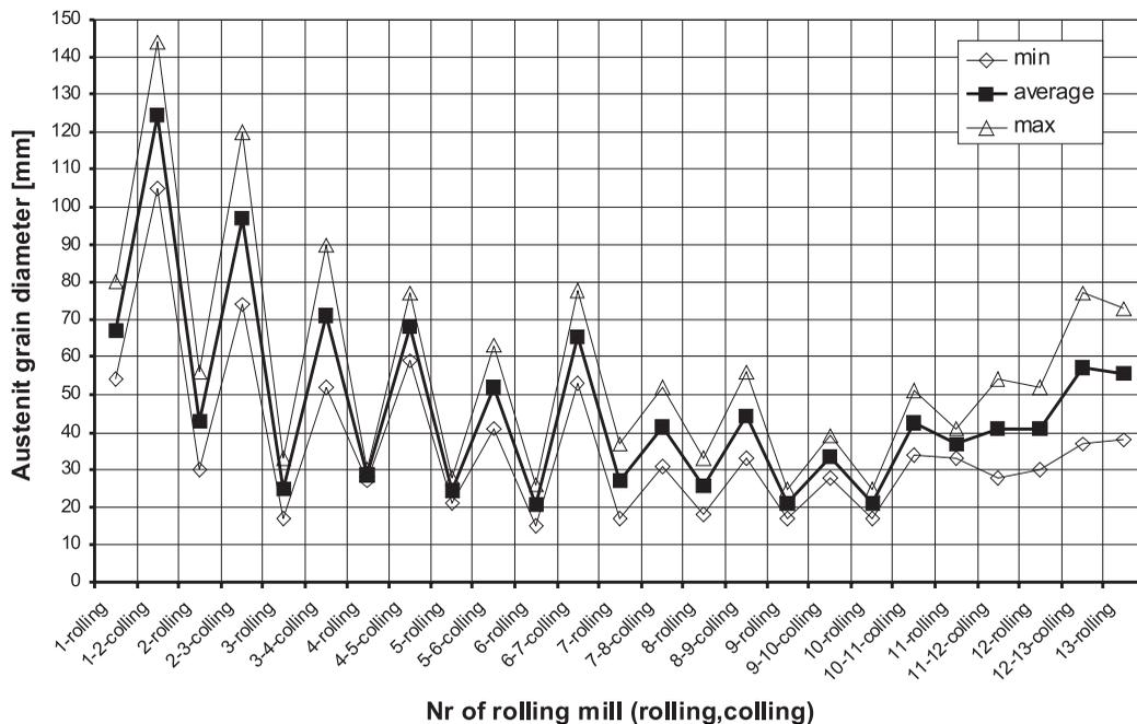
Fig. 4. Austenite grain size variation during rolling 50x20 mm flat bars (Variant I – without accelerated cooling in the rolling line)
