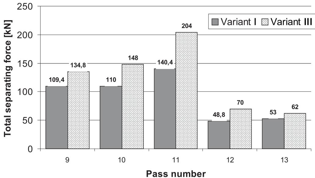
Fig. 7. Total separating force during rolling 50x20 mm flat bars for Variant I and Variant III
