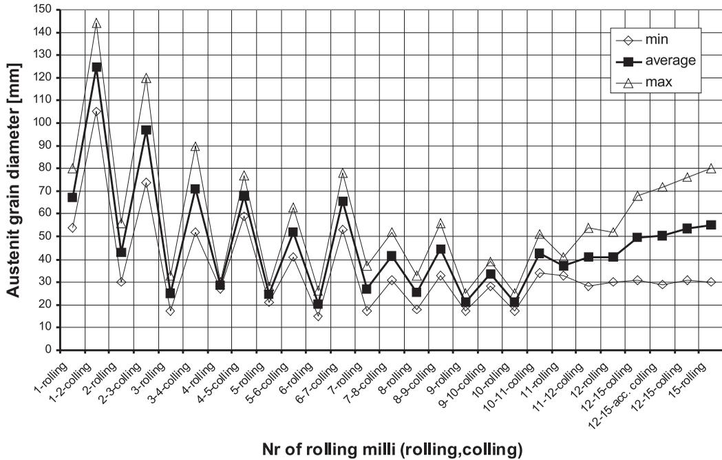
Fig. 5. Austenite grain size variation during rolling 50x20 mm flat bars (Variant II – with one accelerated strip cooling in the rolling line)
