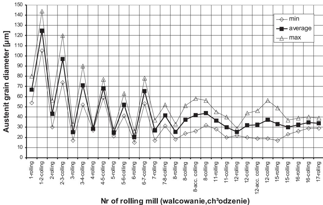
Fig. 6. Austenite grain size variation during rolling 50x20 mm flat bars (Variant II – with two accelerated strip cooling in the rolling line)
