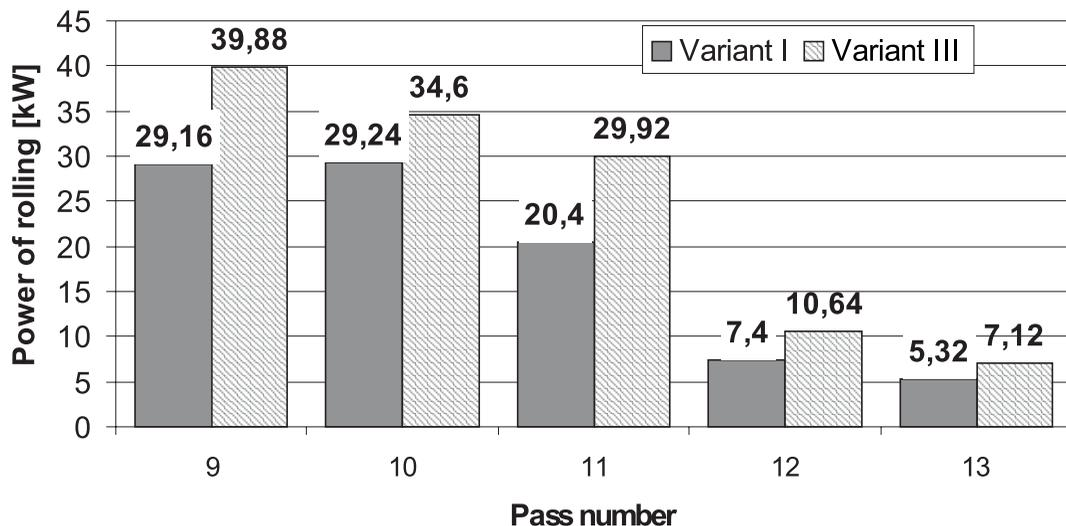
Fig. 8. Power of rolling during rolling 50x20 mm flat bars for Variant I and Variant III
