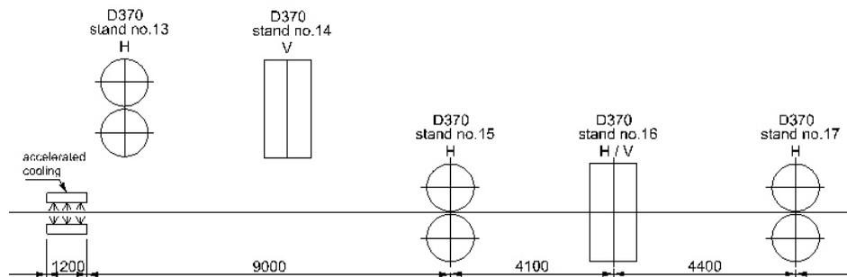
Fig. 3. Scheme of rolling 50x20 mm flat bars with two accelerated cooling section applied: a) intermediate group, b) finishing group – Variant III
