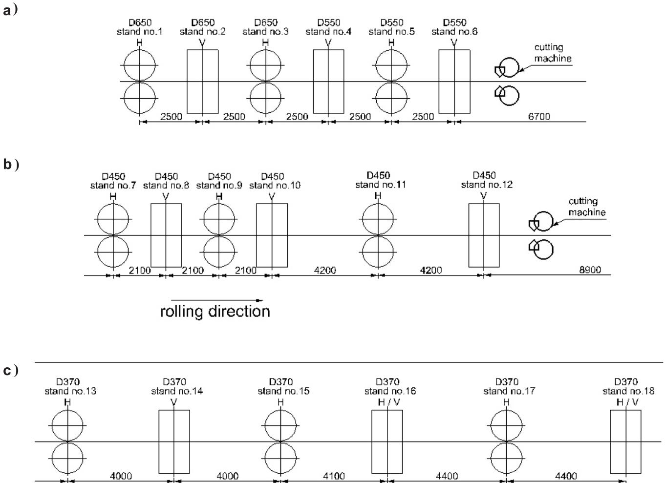
Fig. 1. Scheme of rolling 50x20 mm flat bars without accelerated strip cooling in the rolling line: a) roughing group, b) intermediate group, c) finishing group – Variant I
