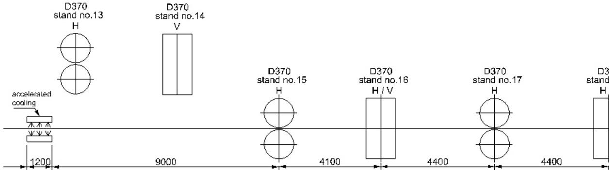
Fig. 2. Scheme of rolling 50x20 mm flat bars with one accelerated cooling section applied: a) intermediate group, b) finishing group – Variant II
