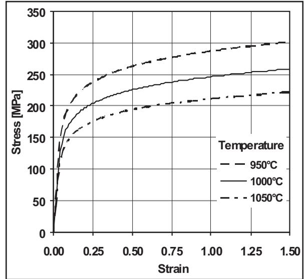
Fig. 3. Rheological properties: a) steel C45, b) steel 306L
