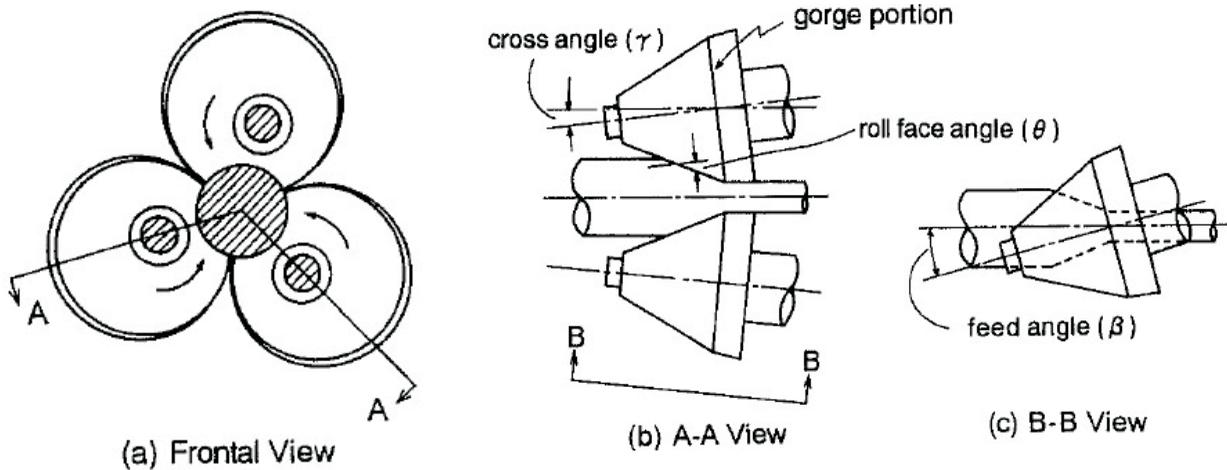
Fig. 1. Scheme of round bimetallic bar rolling process [2]
