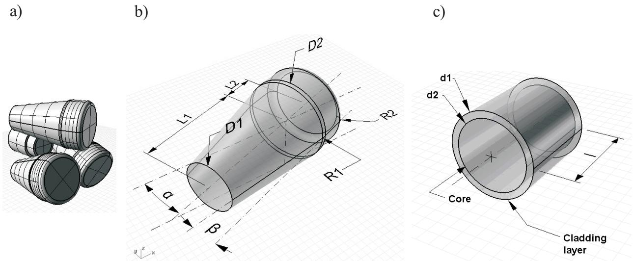
Fig. 2. Shape of the object used in numerical modeling: a) position of rolls, b) roll dimensions, c) bimetallic bar dimensions
