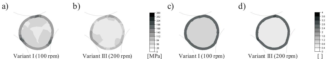
Fig. 9. Distribution of rolling parameters on the sample cross-section: a,b) stress effective, c,d) strain effective
