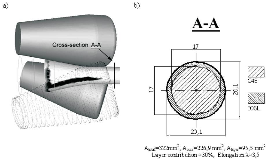
Fig. 4. Results of the numerical modeling: a) shape of bimetallic bar, b) dimensions of the bimetallic bar on cross-section
