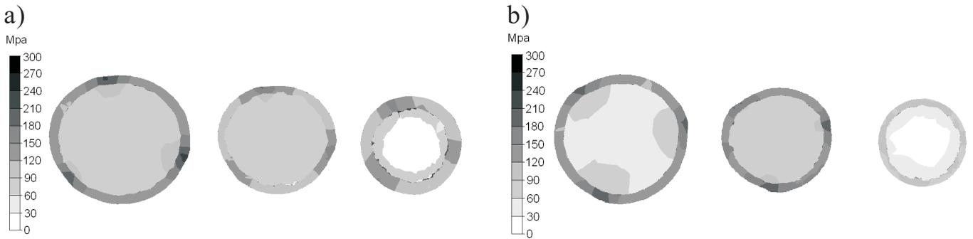
Fig. 6. Distribution of stress effective on the sample cross-section: a) roll diameter 60 mm, b) roll diameter 100 mm
