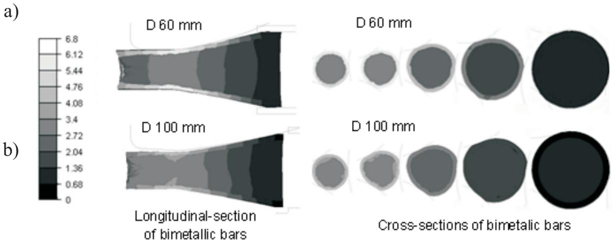
Fig. 7. Distribution of strain effective on the sample cross-section and sample longitudinal-section: a) roll diameter 60 mm, b) roll diameter 100 mm
