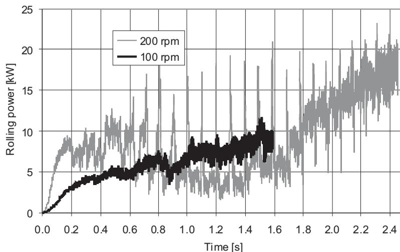
Fig. 10. Distributions of rolling power for rotational speeds: 100 rpm and 200 rpm
