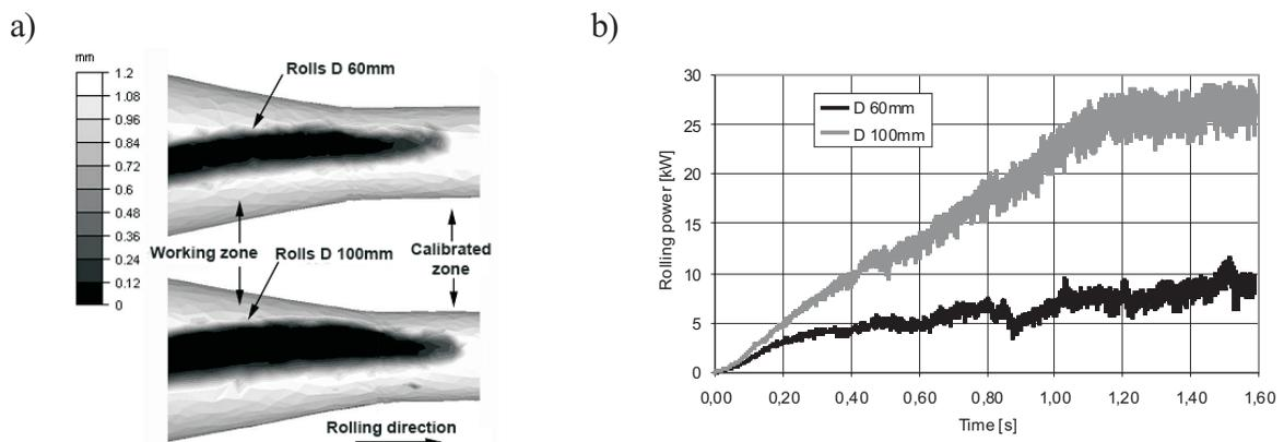
Fig. 5. Results of numerical modeling: a) contact area between sample and rolls, b) distribution of rolling power for two roll diameters
