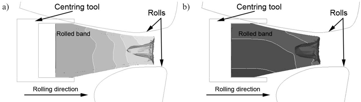
Fig. 8. Distribution of velocity metal flow in the rolling direction on the sample longitudinal-section: a) rotational speed 100 rpm I, b) rotational speed 200 rpm
