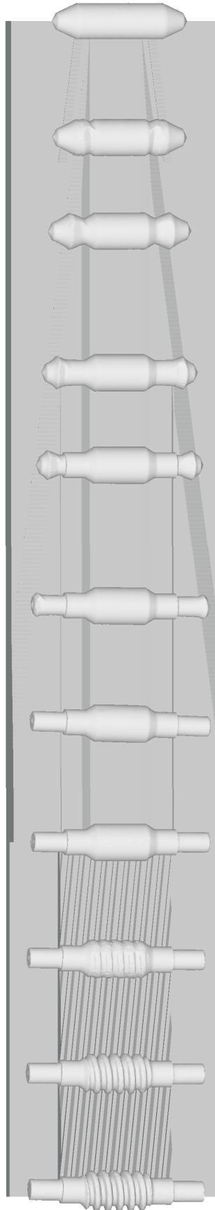
Fig. 10. The shape progression of stepped shaft with worm in analysed process
