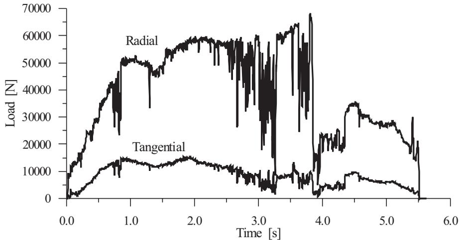
Fig. 12. The loads distribution (calculated by FEM) in rolling process of shaft shown in Fig. 6
