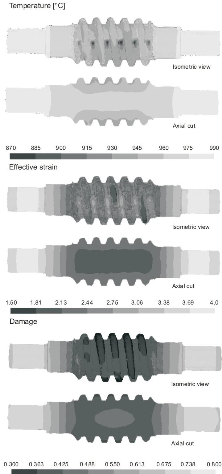
Fig. 11. The temperature, effective strain and Cockroft-Latham damage criterion distributions in stepped shaft with worm
