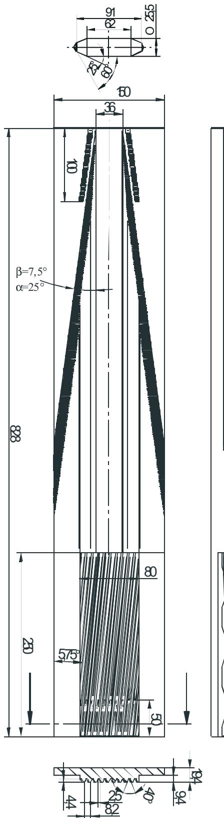
Fig. 8. The billet and wedge tool applied in rolling process of shaft shown in Fig. 6
