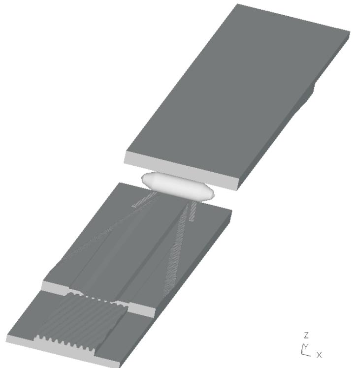
Fig. 9. The geometrical model of CWR process of shaft with worm built in DEFORM-3D software
