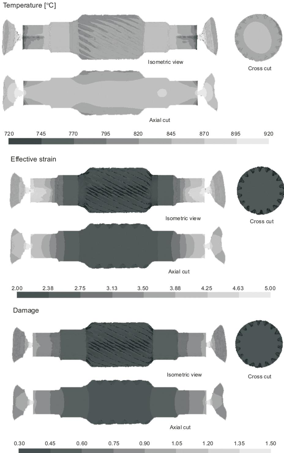
Fig. 5. The temperature, effective strain and Cockcroft-Latham damage criterion distributions in stepped shaft with skew teeth
