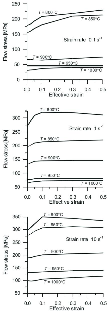
Fig. 3. Flow curves of Ti6Al4V titanium alloy
