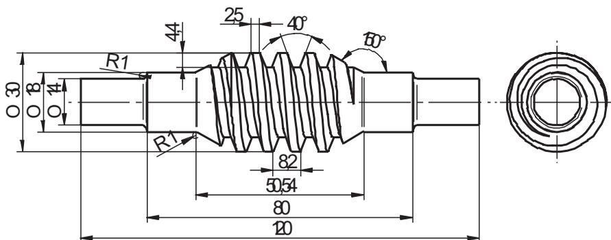
Fig. 7. Stepped shaft with worm
