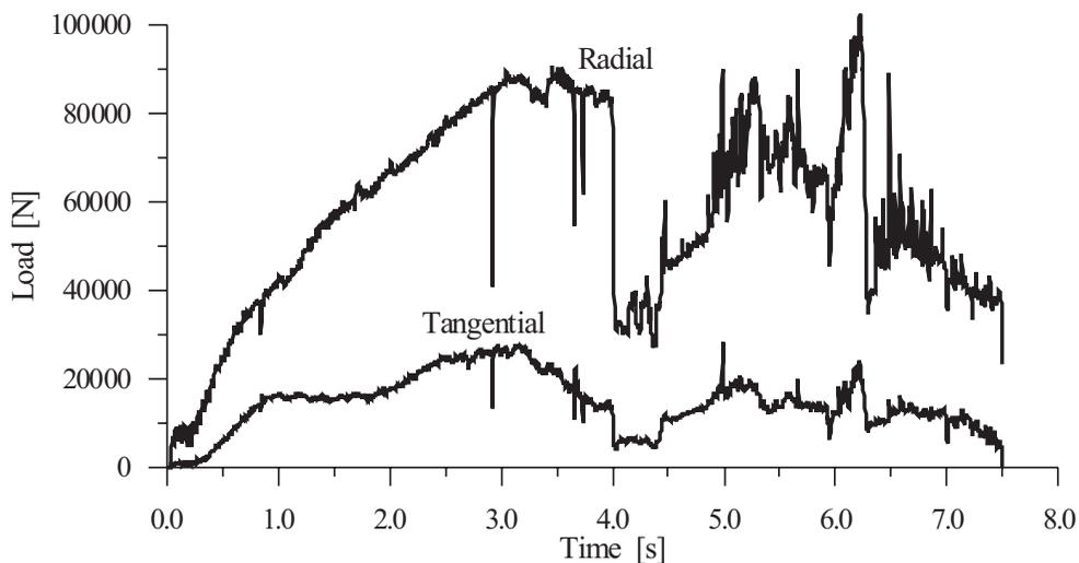
Fig. 6. The loads distributions in CWR process of toothed shaft shown in Fig. 1
