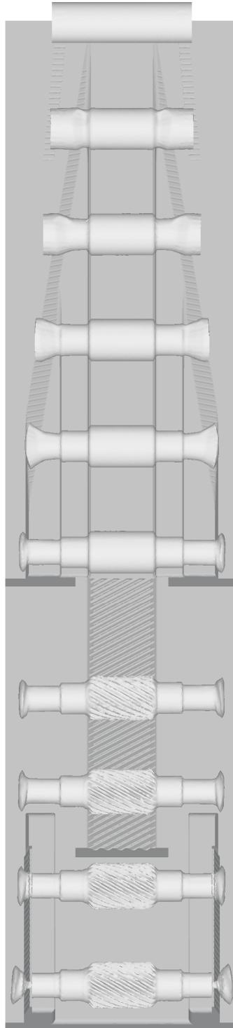
Fig. 4. The shape progression of toothed shaft rolled by means of tools shown in Fig. 2
