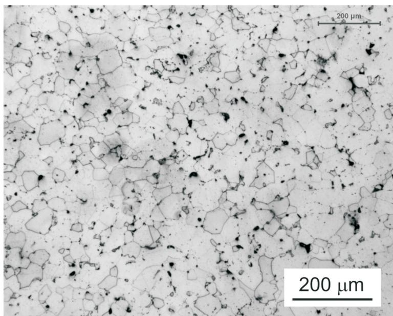
Fig. 5. The typical microstructure of the E steel
