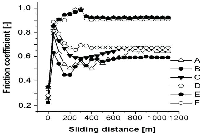
Fig. 7. The variation of friction coefficient measured during the dry sliding tests conducted at the applied normal load of 5 N
