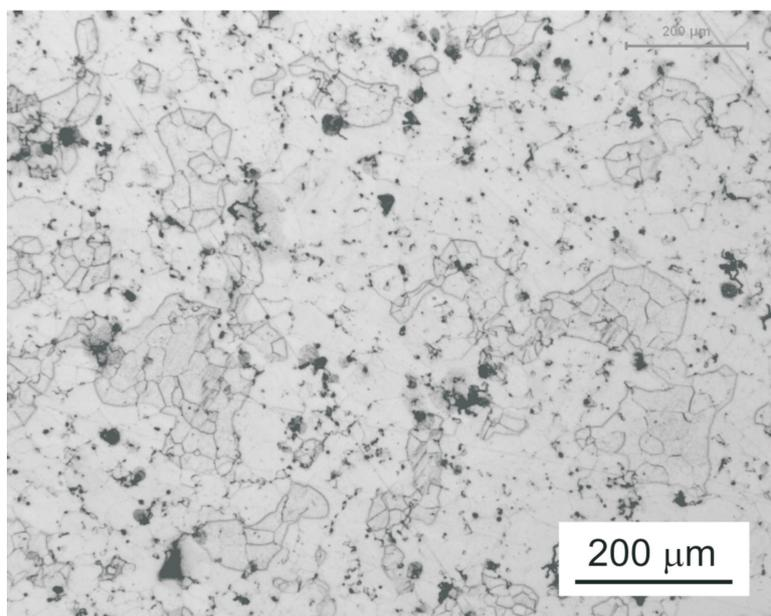
Fig. 6. The typical microstructure of the F steel
