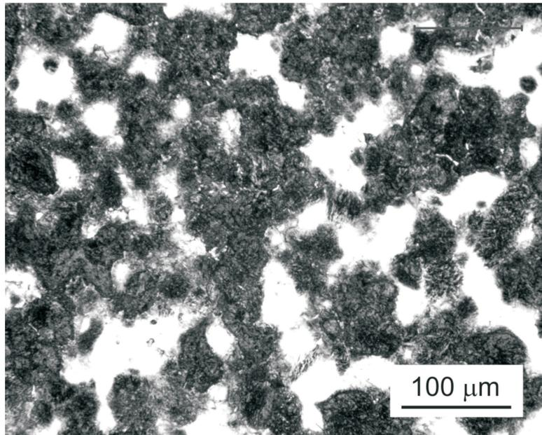
Fig. 3. The typical microstructure of the C steel
