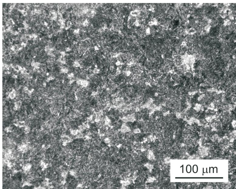
Fig. 1. The typical microstructure of the A steel
