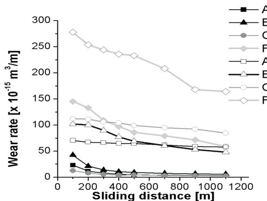
Fig. 10. The wear rate at the applied normal load of 5 N and 10 N
