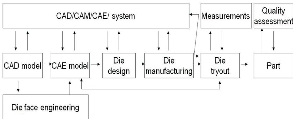
Fig. 2. A product development process with CAD/CAM/CAE system support
