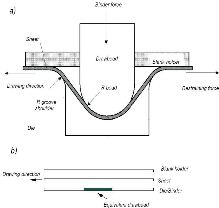
Fig. 14. Drawbead models: (a) geometrical, (b) equivalent
