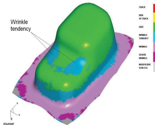
Fig. 8. Final shape of a bathtub 1200 S for the initial die design
