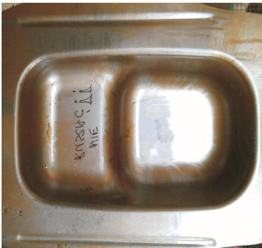
Fig. 20. The example photo of bathtub 1200 S before trimming operation
