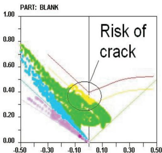
Fig. 12. The minor and major strain and Forming Limit Diagram (FLD) (blank holder pressure 4.0 MN)
