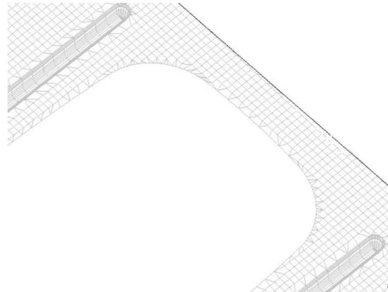
Fig. 13. The geometrical FEM drawbead model
