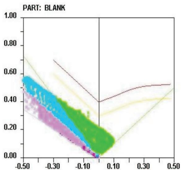
Fig. 9. The minor and major strain and Forming Limit Diagram (FLD) for the initial die design
