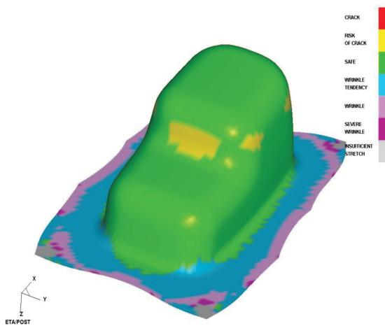
Fig. 11. Final shape of a bathtub 1200 S (blank holder pressure 4.0 MN)
