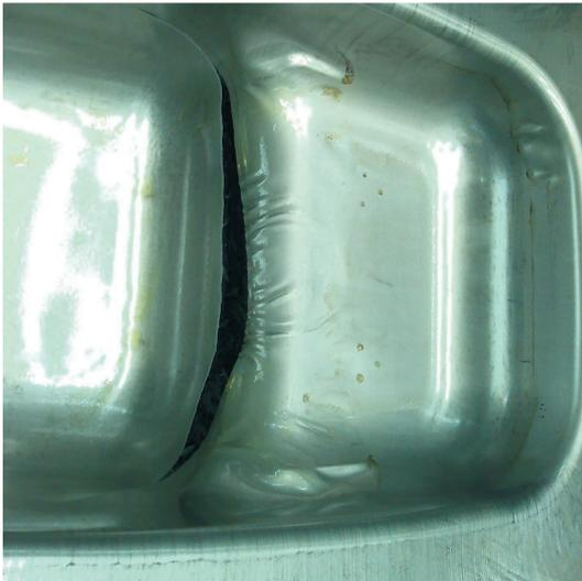
Fig. 4. The split and wrinkles localization after stamping process of bathtub 1200 S
