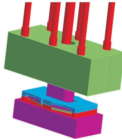
Fig. 7. 3D solid model of drawing die
