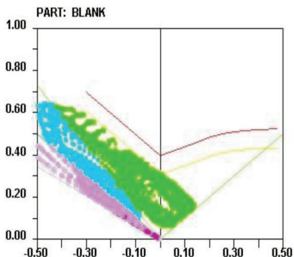
Fig. 19. The minor and major strain and Forming Limit Diagram for the modified die design
