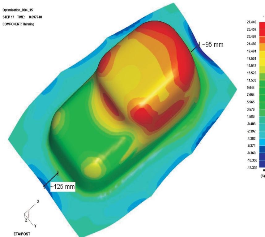
Fig. 17. Thinning distribution for the final part
