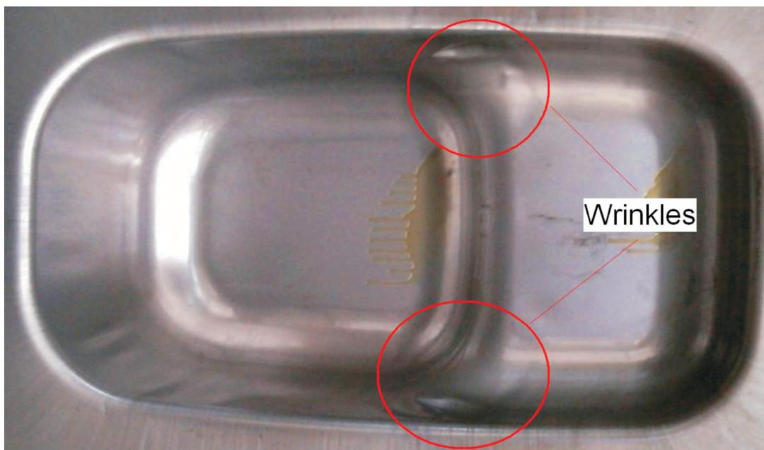
Fig. 10. The wrinkles localization after stamping process of bathtub 1200 S for the initial die design
