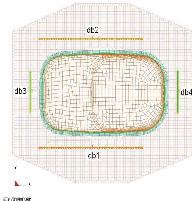
Fig. 15. Drawbead distribution on the die face
