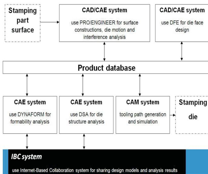
Fig. 5. The scheme of the integrated CAD/CAM/CAE/IBC system of stamping part
