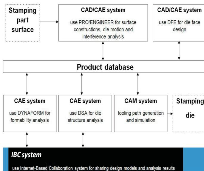
Fig. 5. The scheme of the integrated CAD/CAM/CAE/IBC system of stamping part
