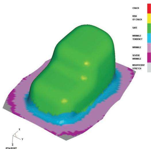
Fig. 18. Final shape of a bathtub 1200 for the modified die design
