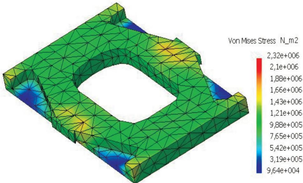
Fig. 21. Equivalent stress distribution for the low ring of the drawing die
