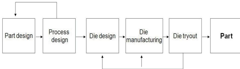
Fig. 1. A traditional process of part development (sequential engineering)
