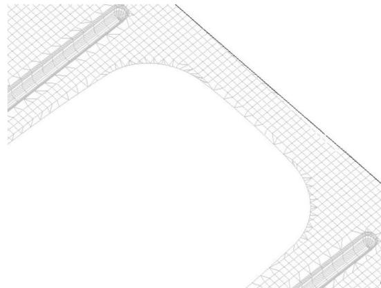
Fig. 13. The geometrical FEM drawbead model
