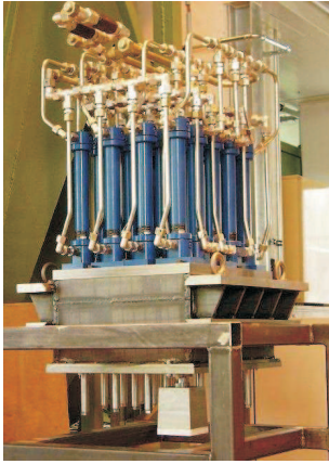
Fig. 6. Multiple stamp press device with hydraulic control
