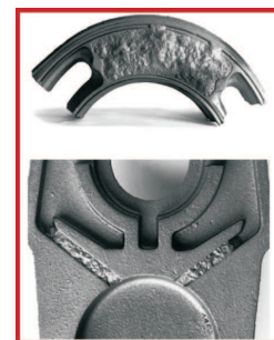
Fig. 2. Cog break at the mould caused by lifting of flask from the pattern plate
