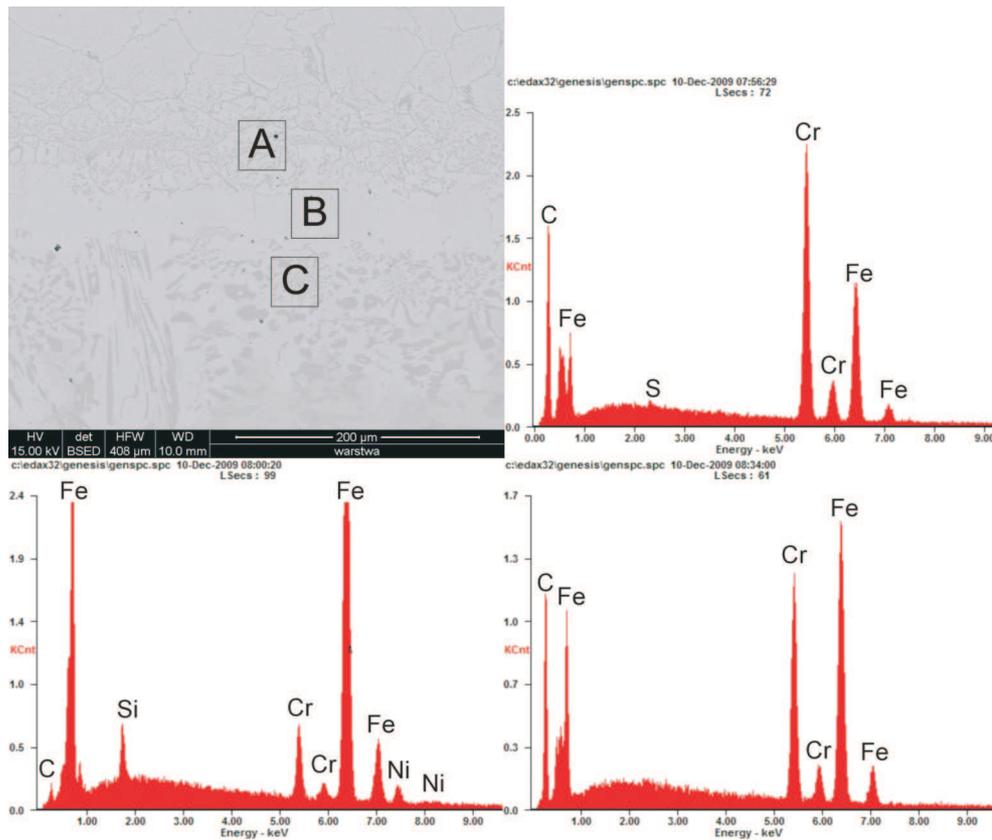
Fig. 8. Distribution of C, Fe, Si, Cr and Ni in transition zone between austenitic steel cast steel and low-alloy cast iron in bimetallic layer casting: a) structure of research area, b) pointwise microanalysis of chemical composition in point "A", c) pointwise microanalysis of chemical composition in point "B", d) pointwise microanalysis of chemical composition in point "C"
