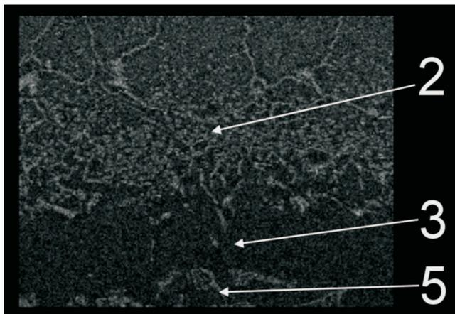
Fig. 10. Superficial distribution of Cr in transition zone between austenitic steel and low-alloy cast iron in bimetallic layer casting. Structure of research area from Fig.8a
