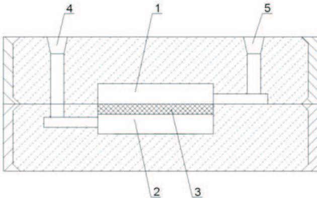
Fig. 1. Technology of bimetallic layer castings with use of two gating systems: 1 – cast iron layer, 2 – cavity (preheater) 3 – steel sheet, 4,5 – gating[6]
