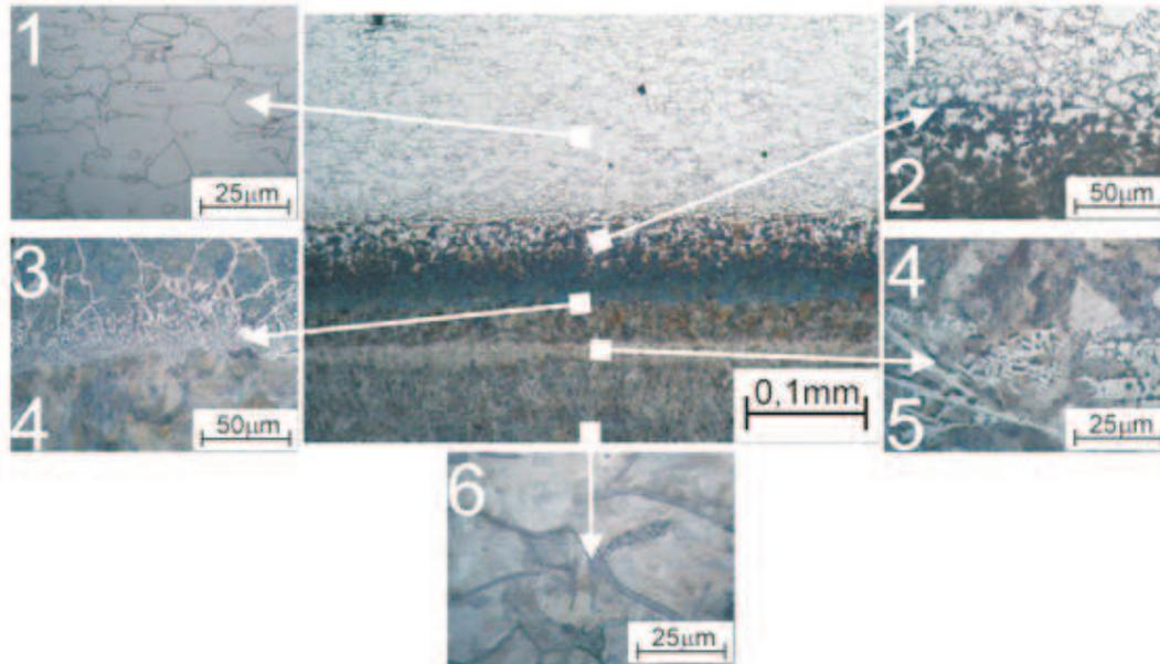
Fig. 5. Microstructure of bimetallic layer casting in configuration: surface layer on the basis of X8Cr 13 ferritic plate of the thickness about 5 mm on low-alloy cast iron EN-GJL-XCr1 base – etching Mi19Fe
