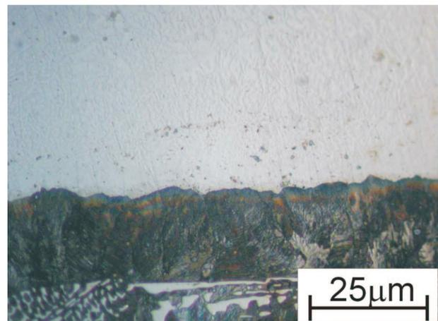
Fig. 9. Microstructure of joint zone in bimetallic layer casting in configuration: austenitic steel plate – low-alloy cast iron. In direction from surface is visible following:  $\alpha + \gamma$ , pearlite, ledeburite + pearlite – etching Mi19Fe
