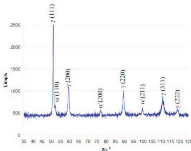
Fig. 7. X-ray diffraction of bimetallic casting with enriched surface by austenitic steel plate after one cycle exploitation in conditions of abrasive action of type metal-mineral
