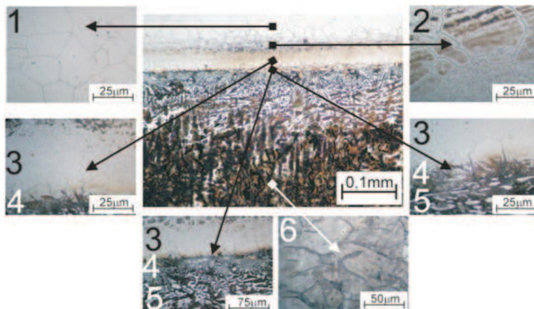
Fig. 6. Microstructure of bimetallic layer casting in configuration: surface layer on the basis of X10CrNi 18-8 austenitic steel plate about thickness  $g = 5$  mm on low-alloy cast iron EN-GJL-XCr1 base – etching Mi19Fe
