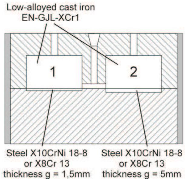
Fig. 2. Section of the sand mould ready to be poured by liquid alloy
