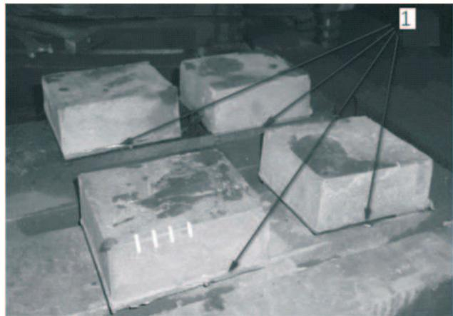
Fig. 3. View of cast iron test-castings with the surface enriched by alloy steel plate – 1
