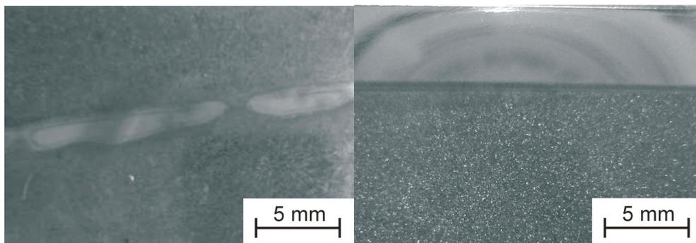
Fig. 4. View of cross-section of bimetallic low-alloy cast iron casting with enriched surface by austenitic steel plate about thickness 1,5mm (a) and 5mm (b)
