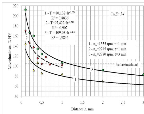
Fig. 9. Hardness measured in layers of CuZn 34 samples, depending on rpm speed of the upper rotor and the treatment time
