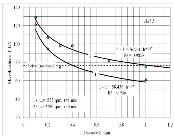
Fig. 8. Hardness measured in layers of AM5 samples, depending on rpm speed of the upper rotor and the treatment time
