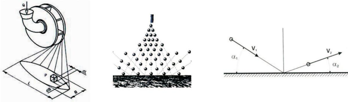
Fig. 1. Schematic diagram of abrasive grain impacting on the surface to be cleaned [7, 8]
