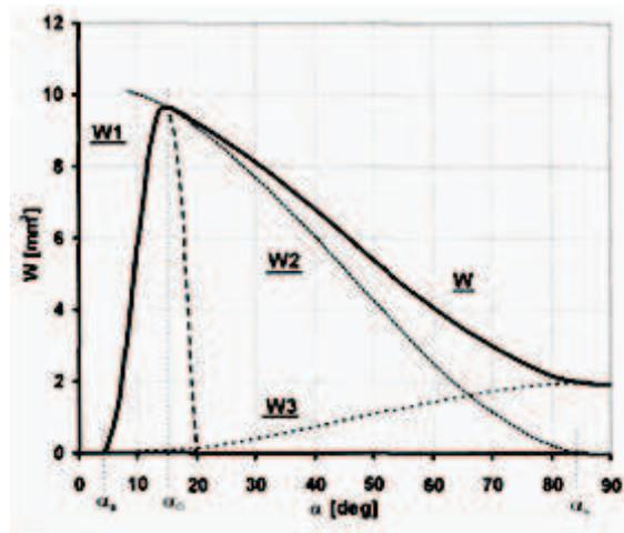
Fig. 2. Component functions of the erosion treatment for soft materials, according to Bitter
