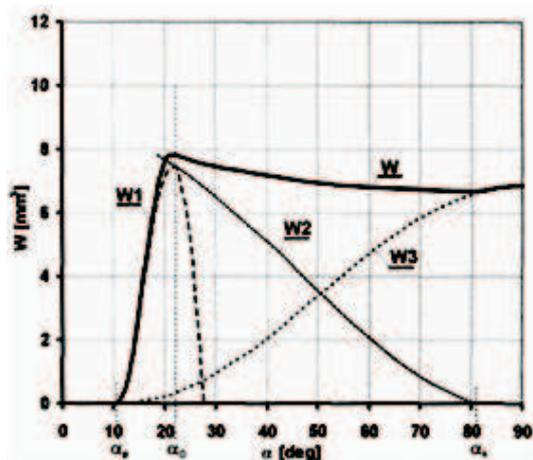
Fig. 3. Component functions of the erosion treatment for hard materials, according to Bitter
