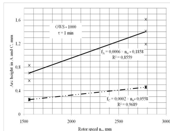
Fig. 6. Intensity of shot stream depending on treatment time and on the rotor speed
