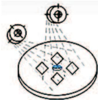
Fig. 5. Layout of rotors with respect to the rotary bench in the shot blasting machine OWS-1000
