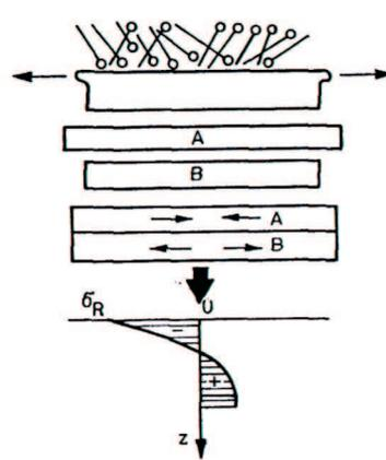
Fig. 4. Model of compressive stress generation as a result of shot-peening process [8]: a – hard materials  $HV > 600$ ; b – plastic ( $HV < 300$ ); a) the pressure effect in accordance with the Hertz model, b) the effect of plastic deformation of the surface layer
