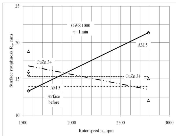
Fig. 7. The change of surface roughness of shot-peened samples made of AM5 and CuZn34 in relation to the rotor rpm speed
