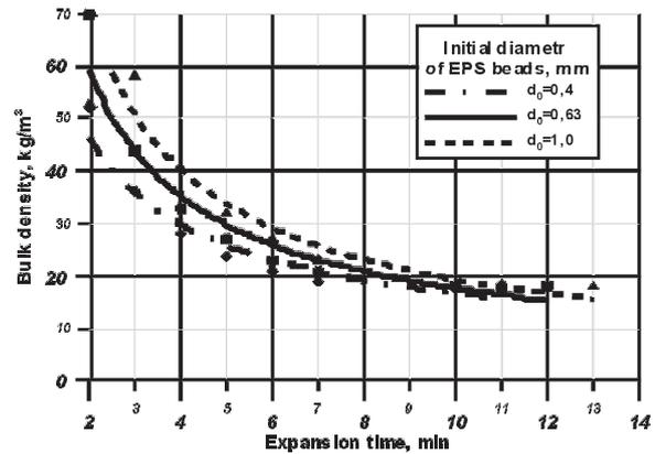
Fig. 2. Dependence of bulk density from the time of expansion and the initial diameter of EPS beads [9]
