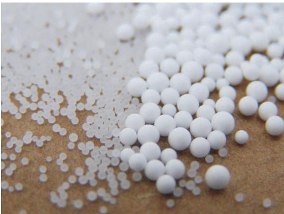
Fig. 1. Beads of polystyrene before and after pre-expansion process
