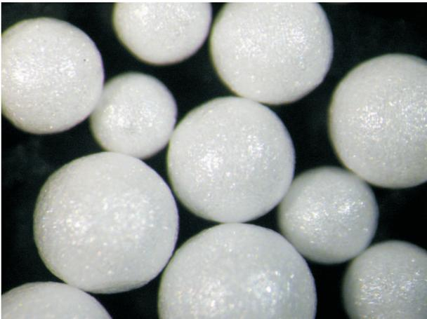
Fig. 8. Beads immediately after expansion, magnification x20
