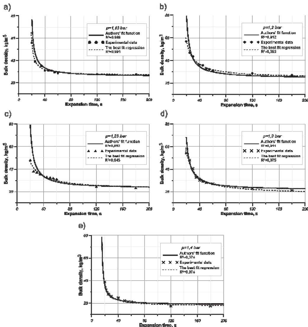
Fig. 7. Effect of expansion time and pressure on the bulk density of foamed polystyrene
