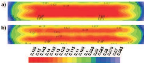
Fig. 4. Distribution of carbon concentration in the cross-section of slab; a)  $V_c=17$ mm/s; b)  $V_c=20$ mm/s
