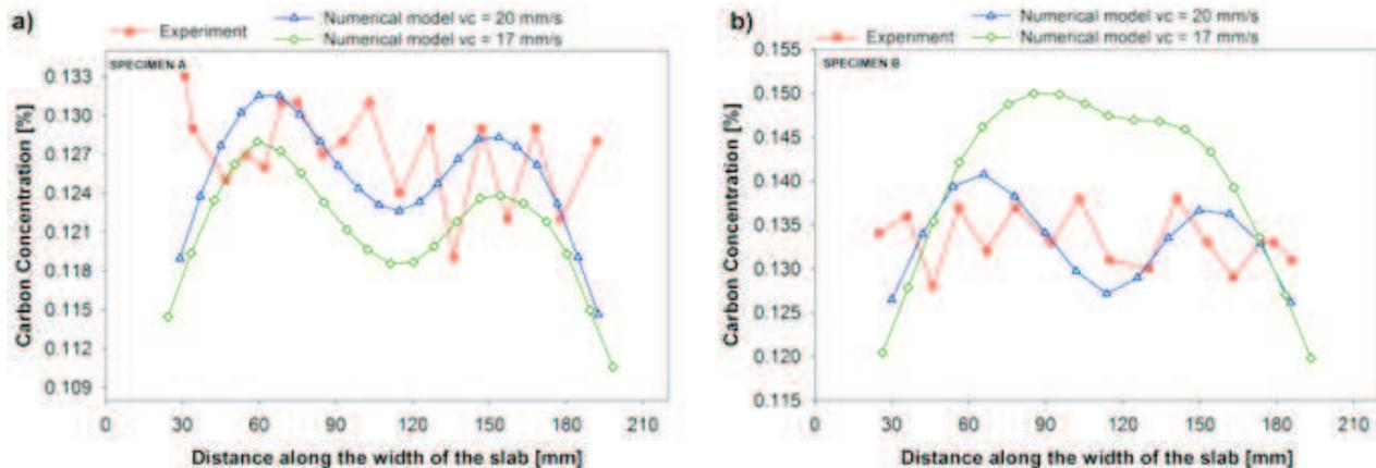
Fig. 5. Carbon concentration along the width of slab; a) centre; b) surface of slab
