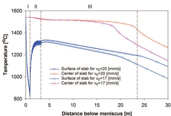
Fig. 2. Change of temperature in slab during continuous casting process
