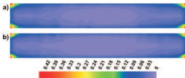
Fig. 6. Distribution of strain intensity in the cross-section in continuous cast billet, after finish of solidification process; a)  $V_c=17\text{mm/s}$ ; b)  $V_c=20\text{mm/s}$
