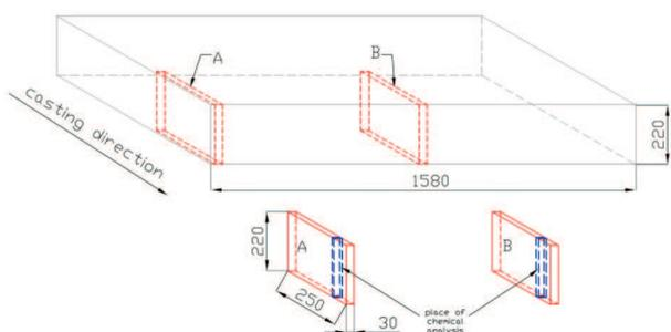
Fig. 1. Schematic illustration of sawing and analyzing of the test specimen
