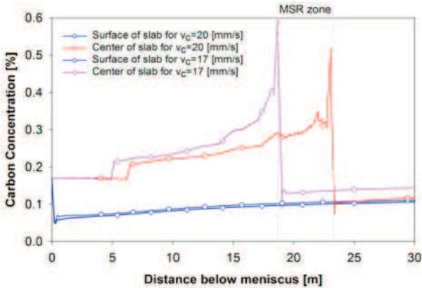
Fig. 3. Change of concentration carbon in slab during continuous casting process
