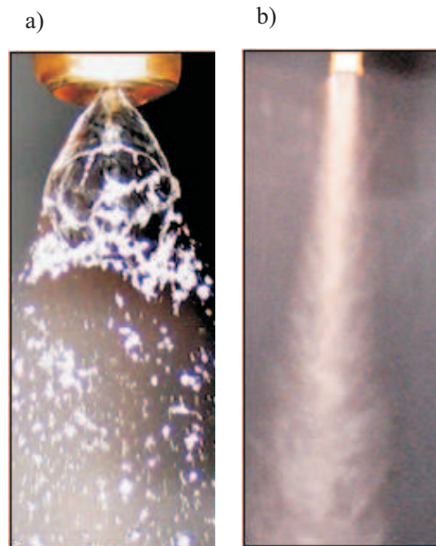
Fig. 2. Stream of sprayed water (a) and water mist (b) obtained with use of designed rotary sprayer
