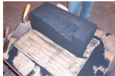
Fig. 5. Part of the mould extracted from moulding box
