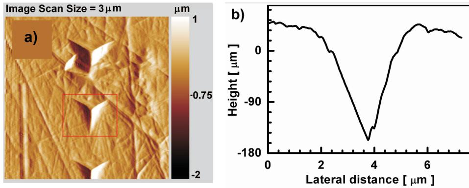
Fig. 1. The indent pattern image (a) and depth profile (b) of PLZT ceramics
