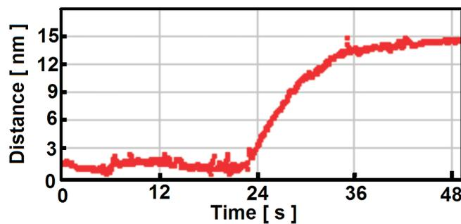
Fig. 2. The dynamics of photostrictive effect of the surface PLZT ceramics
