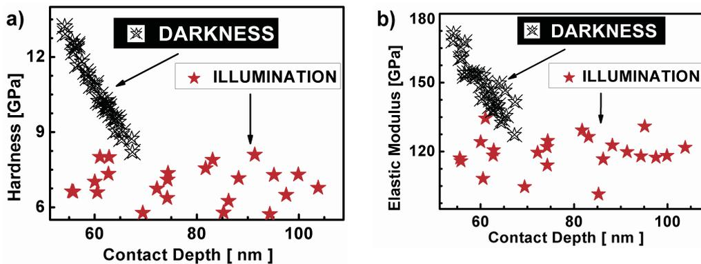
Fig. 3. Hardness(a) and modulus plots(b) of dark (black colour) and illuminated (red colour) PLZT ceramics
