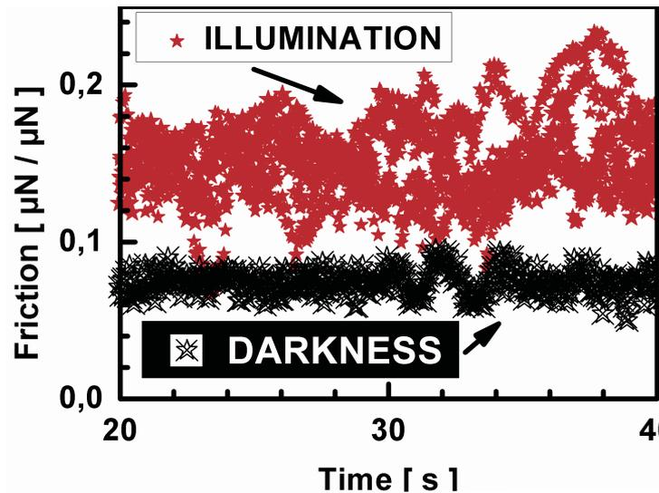
Fig. 4. Friction coefficient of dark and illuminated PLZT ceramics surface
