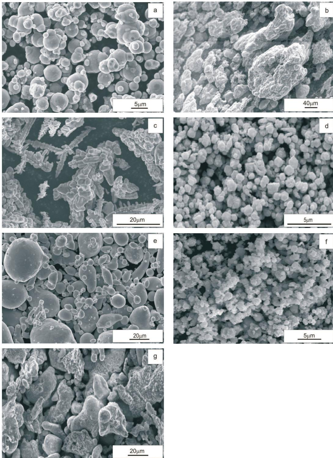
Fig. 1. SEM micrographs of experimental powders: (a) carbonyl iron *Fe CN* (BASF) (b) atomised iron *ABC 100.30* (Höganäs) (c) electrolytic copper *CH-L 10* (ECKA) (d) fine reduced copper *MT 100* (ECKA) (e) atomised tin *30 GN-350* (ECKA) (f) carbonyl nickel *T110* (INCO) (g) atomised tin bronze *85/15 25 GR-325* (ECKA)
