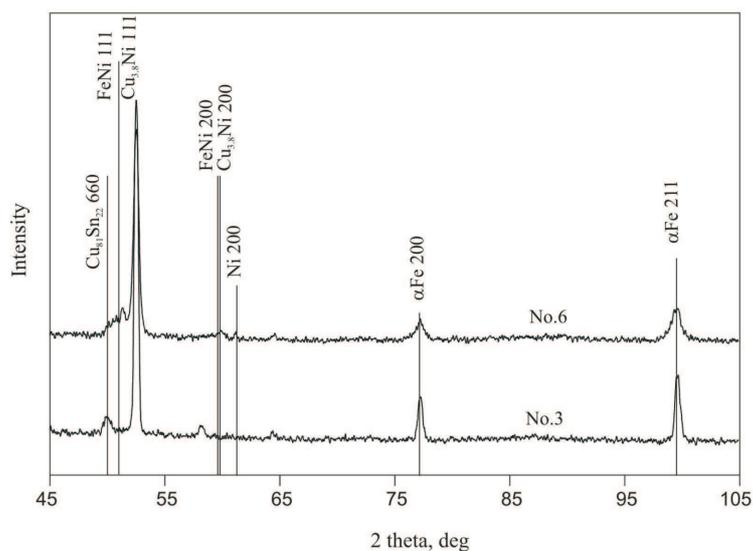
Fig. 5. X-ray diffraction patterns of materials No. 3 (85% *Fe CN* + 15% 25 *GR-325*) and No. 6 (75% *Fe CN* + 15% 25 *GR-325* + 10% *T110*)
