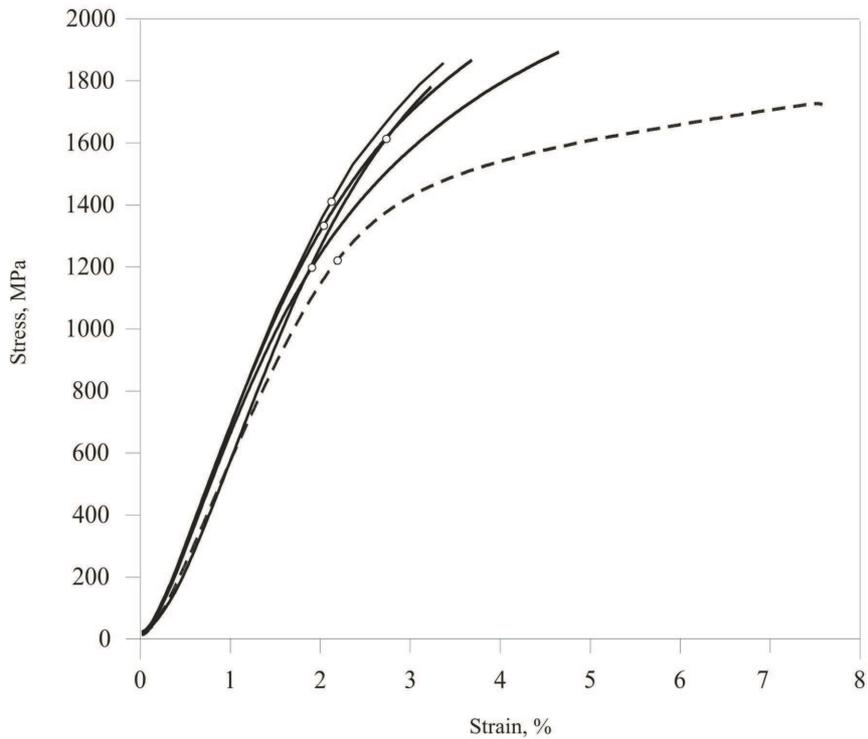
Fig. 3. The stress-strain behaviour of material No. 6 (solid curves) and hot pressed cobalt (dashed curve). White dots indicate the 0.2% offset yield strength
