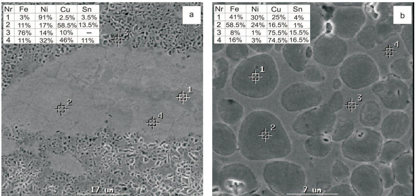
Fig. 6. Examples of electron probe micro analysis carried out in selected areas of a metallographic specimen of material No. 6
