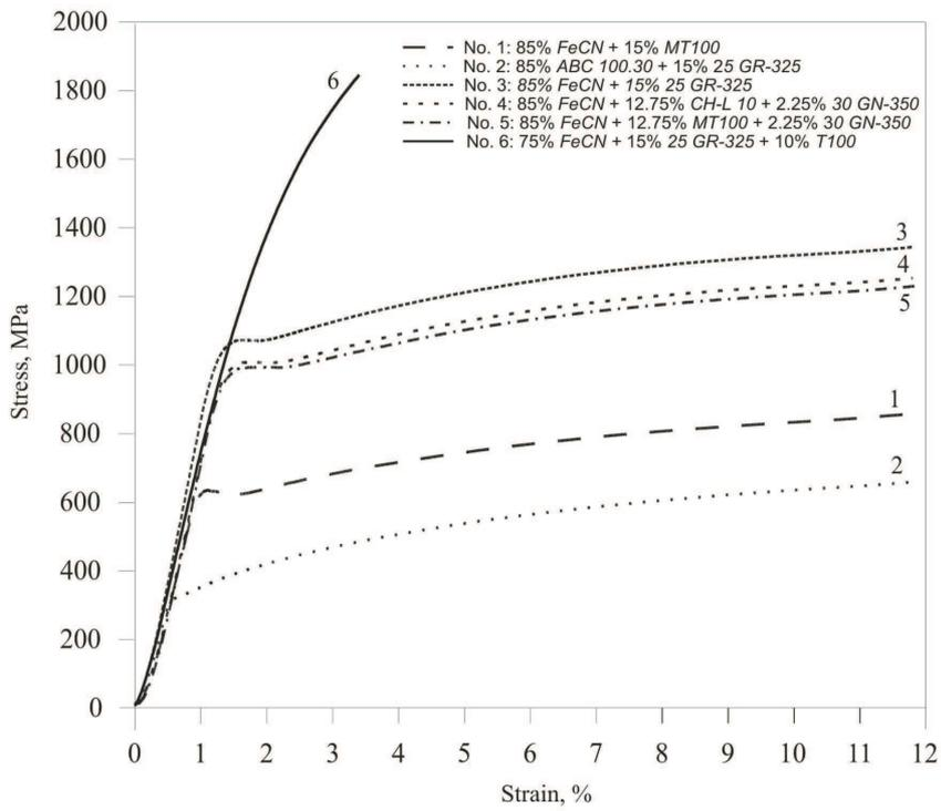
Fig. 2. The stress-strain behaviour of the investigated materials under 3-point bending conditions
