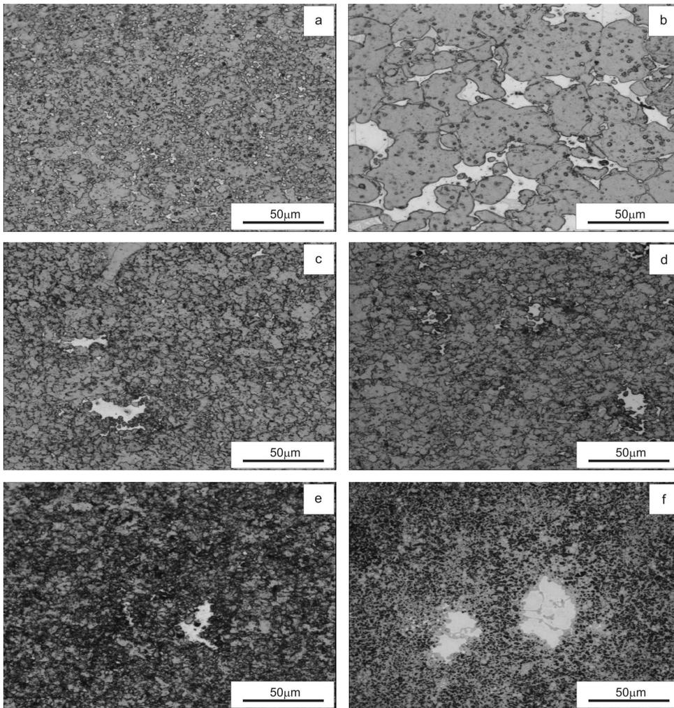
Fig. 4. LM microstructures of selected specimens hot pressed of: (a) 85% *Fe CN* + 15% *MT 100* (No.1) (b) 85% *ABC 100.30* + 15% 25 *GR-325* (No.2) (c) 85% *Fe CN* + 15% 25 *GR-325* (No.3) (d) 85% *Fe CN* + 12.75% *CH-L 10* + 2.25% 30 *GN-350* (No.4) (e) 85% *Fe CN* + 12.75% *MT 100* + 2.25% 30 *GN-350* (No.5) (f) 75% *Fe CN* + 15% 25 *GR-325* + 10% *T110* (No.6)
