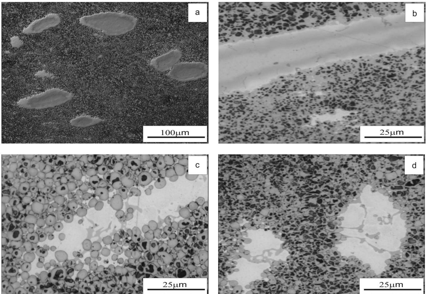
Fig. 7. LM micrographs showing microstructures in various areas of a metallographic specimen of material No. 6: (a) inclusions of nickel and copper-rich phases in an iron-rich matrix (b) large plate-like inclusion with a nickel-rich core (c) rounded iron and nickel-rich inclusions formed in abundant liquid (as in Figure 6b) (d) fibrous nickel-rich phase (grey) within a copper-rich lakes (as in Figure 6a)
