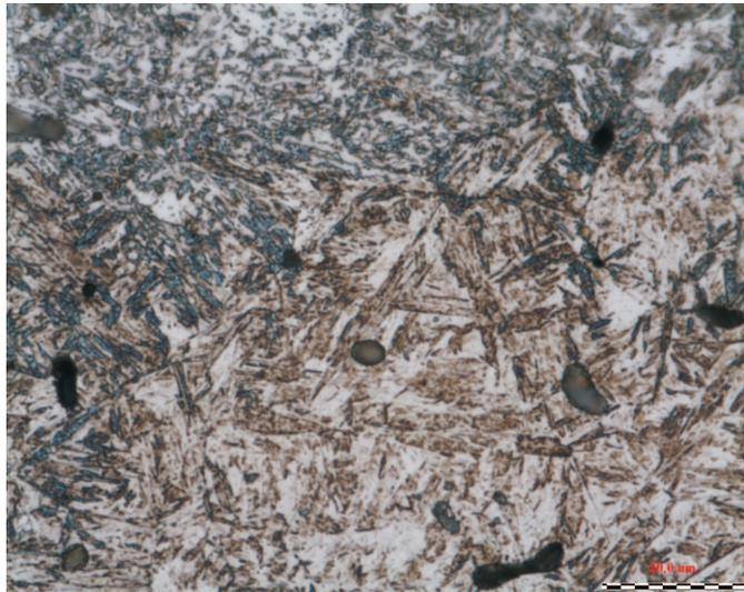
Fig. 3. Microstructure of 3%Mn+CrL+0.3%C steel; ST=1250°C, 100%N<sub>2</sub>; M, B, A
