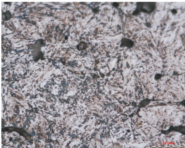
Fig. 5. Microstructure of 3%Mn+CrM+0.3%C steel; ST=1250°C, 100%N<sub>2</sub>; B, M, pores
