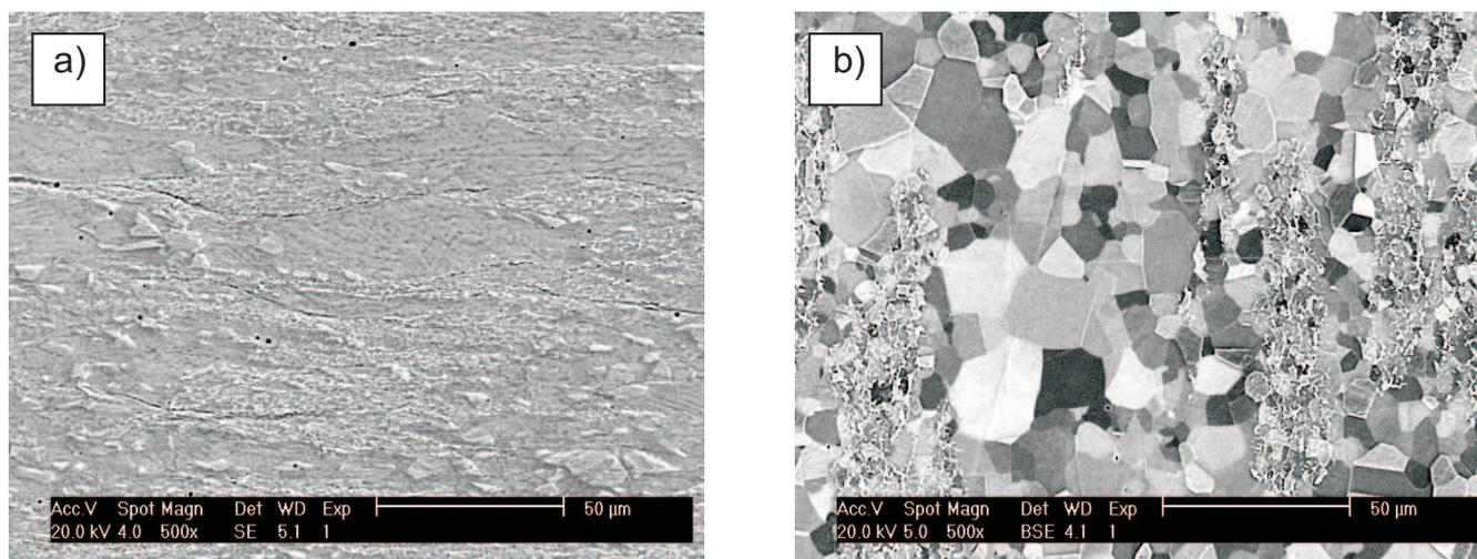
Fig. 1. Microstructure of  $\text{Ni}_3\text{Al}$  foils, (a) after rolling, (b) after rolling and a heat treatment at  $1000^\circ\text{C}$  in two hours
