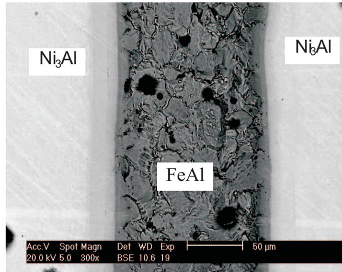
Fig. 6. Microstructure of Ni<sub>3</sub>Al/FeAl/Ni<sub>3</sub>Al joint after high-current pulses sintering
