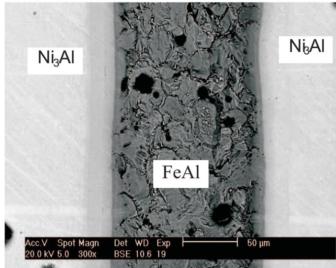
Fig. 6. Microstructure of  $\text{Ni}_3\text{Al}/\text{FeAl}/\text{Ni}_3\text{Al}$  joint after high-current pulses sintering
