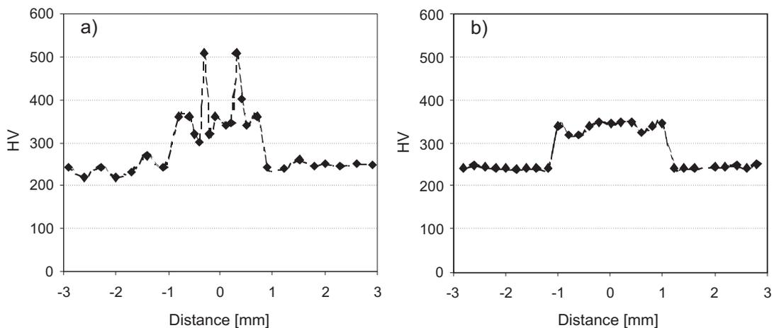
Fig. 5. Linear microhardness measurements of  $\text{Ni}_3\text{Al}/\text{FeAl}/\text{Ni}_3\text{Al}$  joint, (a) variant I, (b) variant II
