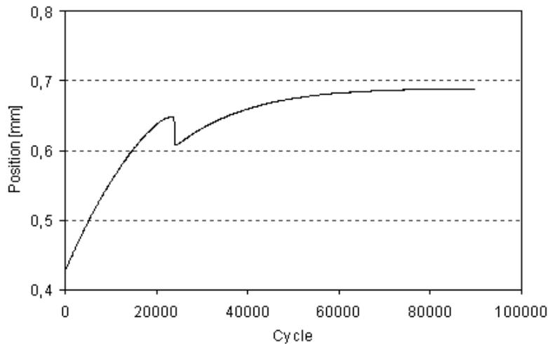
Fig. 2. Influence of SHS reaction on lower stamp position during presintering process
