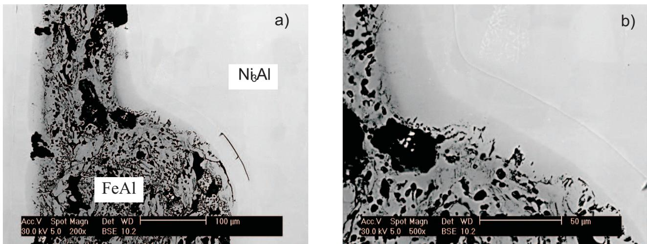
Fig. 3. Microstructure of  $\text{Ni}_3\text{Al}/\text{FeAl}/\text{Ni}_3\text{Al}$  joint (variant I), (a) local cracks along the boundary  $\text{Ni}_3\text{Al}$  - first transient zone, (b) transient zones
