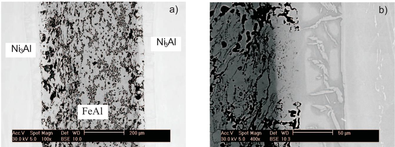
Fig. 4. Microstructure of  $\text{Ni}_3\text{Al}/\text{FeAl}/\text{Ni}_3\text{Al}$  joint (variant II), (a) overall view, (b) transient zones
