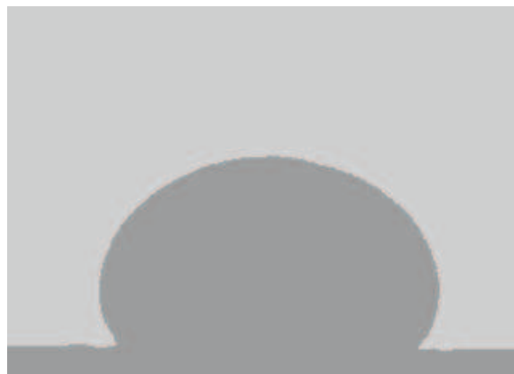
Fig. 1. An alloy drop of 70 wt % Cu, 25 wt % Pb, 5 wt % Fe at 1373 K
