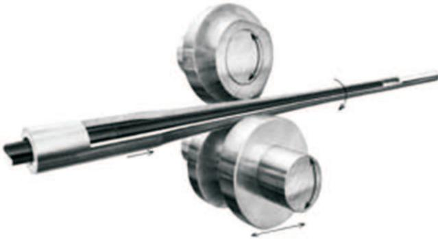
Fig. 1. Conventional cold tube rolling process realized on the pilger mills
