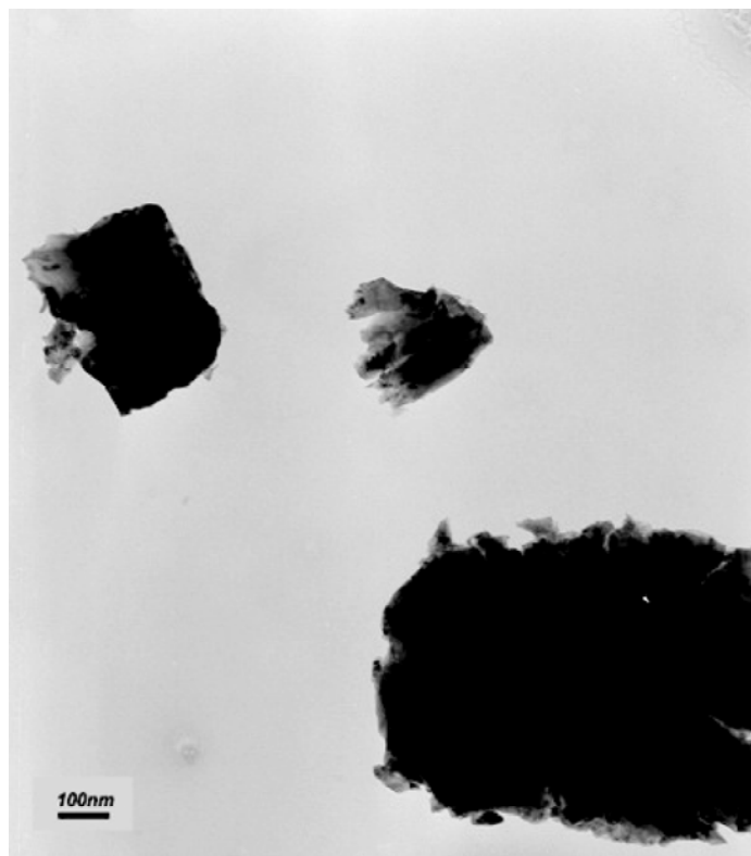
Fig. 5. TEM micrographs of BST60/40 ceramic powder after sintering and milling
