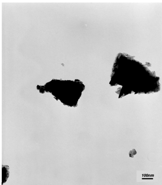
Fig. 6. TEM micrographs of BST50/50 ceramic powder after sintering and milling
